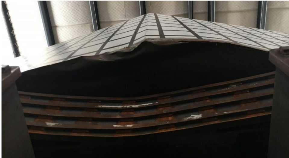
Figure 26. CEM locomotive damage
