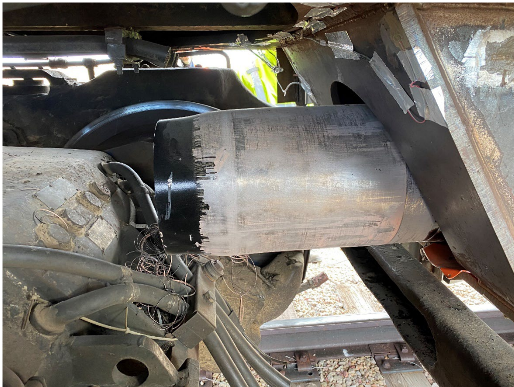
Figure 69. The PBC deformation tube was expanded along its entire stroke of 21”
