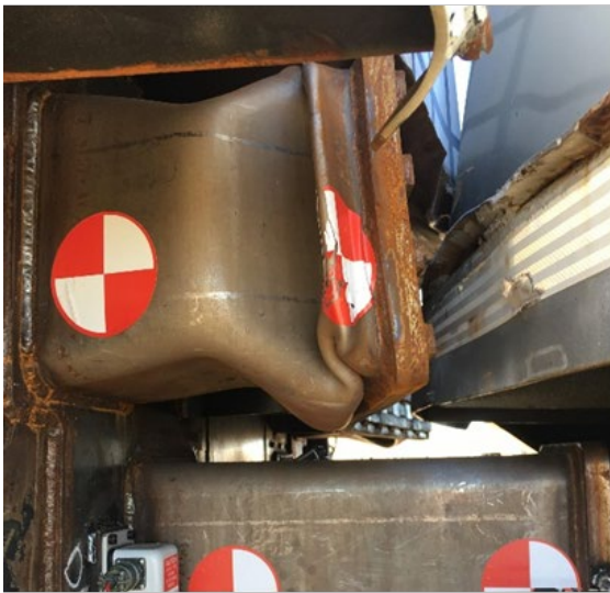
Figure 25. Deformed upper DAC tubes, right and left sides, respectively
