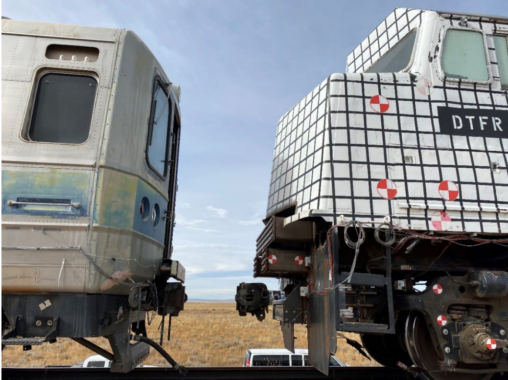
Figure 63. Pre-test photo of the impact interface
