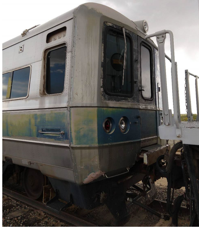
Figure 54. Buffer beam at forward end of M1 cab car selected for VTVT2
