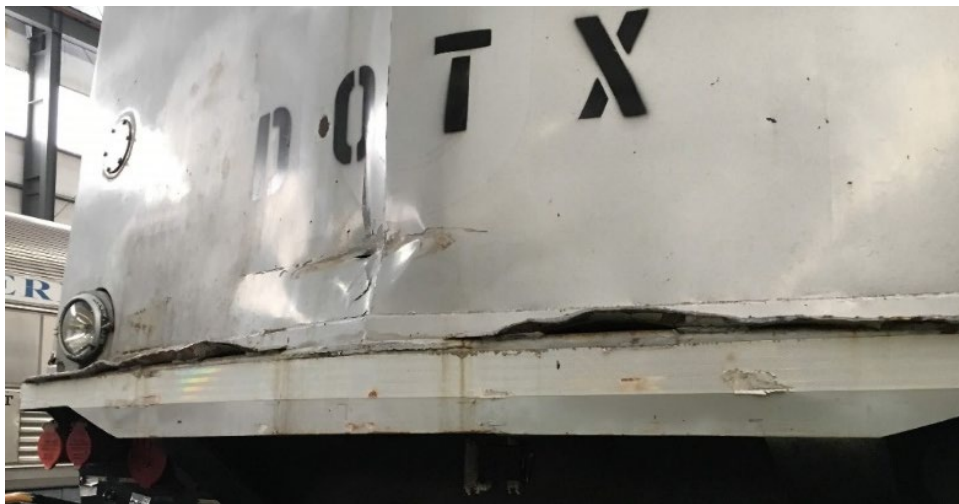
Figure 28. Close-up of conventional locomotive damage
