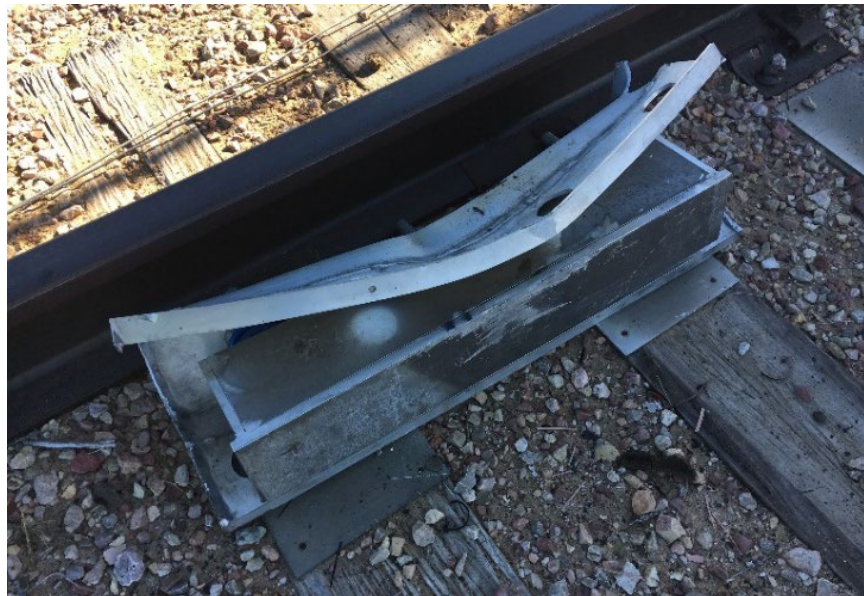
Figure 16. Post-test photograph showing the coupler carrier lying on the track
