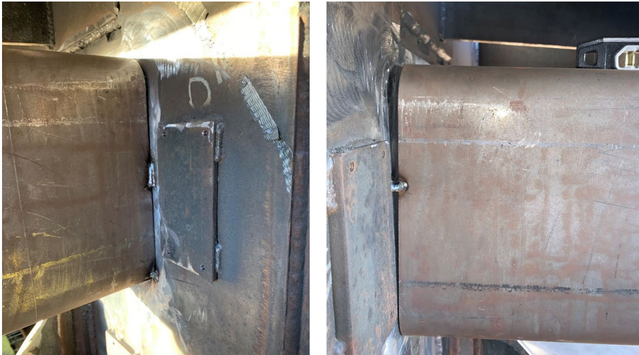
Figure 74. Post-impact deformation of bottom DAC tubes support plate, left (left) and right (right) sides
