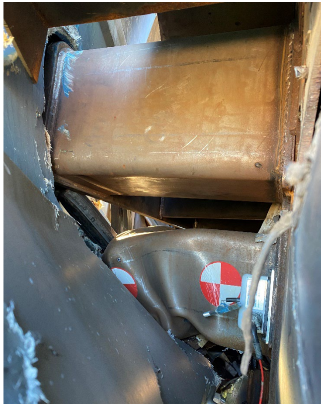
Figure 66. DAC tubes after impact, before the vehicles were separated
