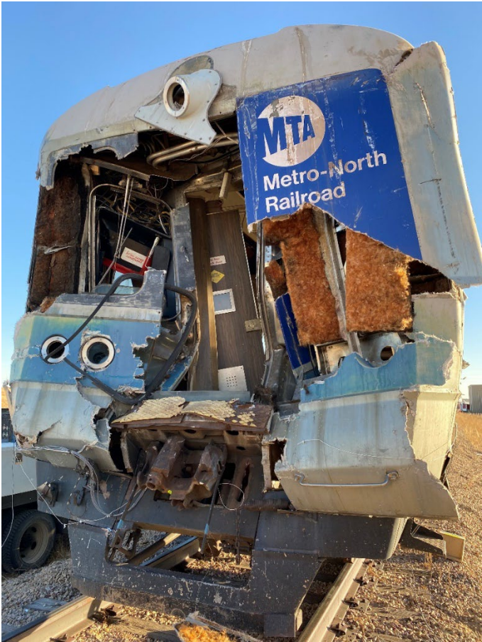
Figure 80. Post-test damage to M1 end frame
