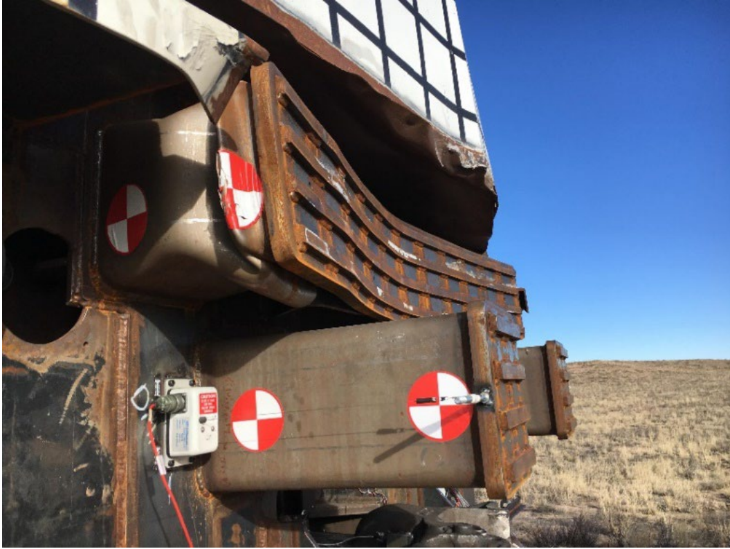
Figure 24. Post-test photograph of DAC showing that only the upper DAC tubes deformed
