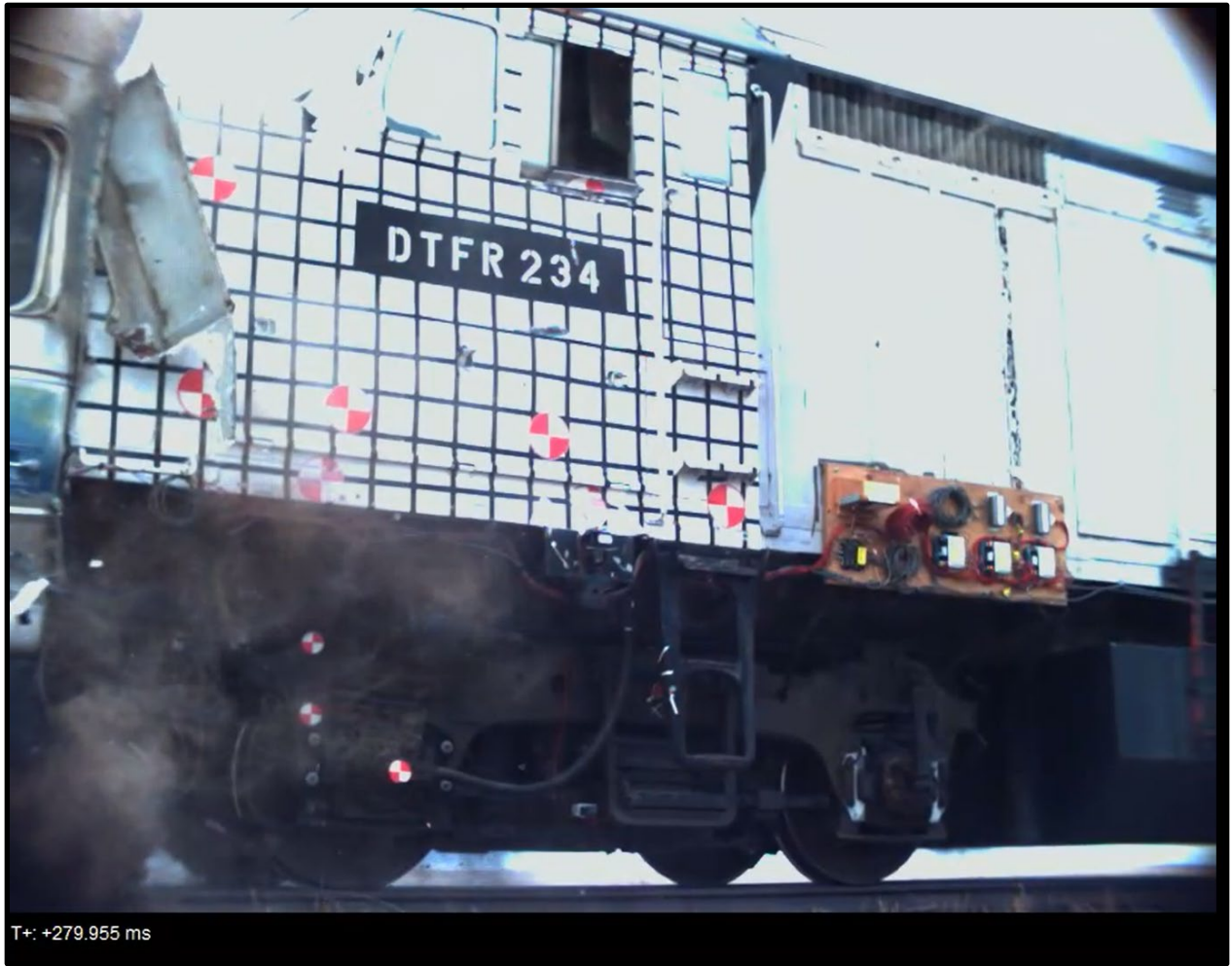
Figure 88. Image taken from a high-speed test video (approximately 280 msec after impact)
