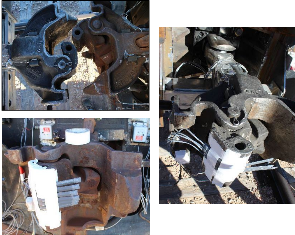
Figure 36. Top Left — a pre-test photograph of the couplers from above; bottom left — impact sensors affixed to the front surface of the stationary conventional locomotive; right — impact sensors affixed to the front surface of the CEM locomotive coupler
