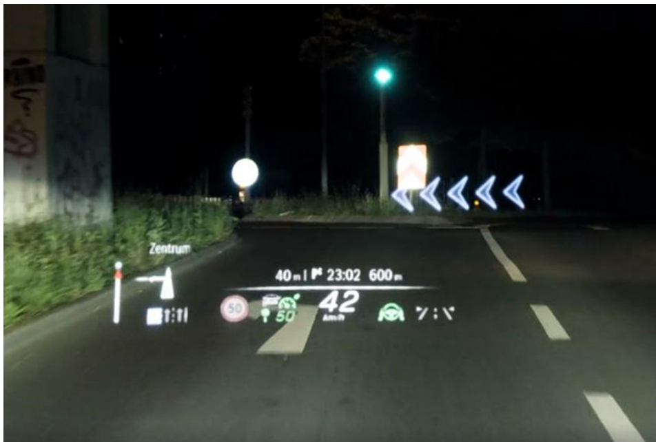
Figure 5 – Example of the AR-HUD for the 2021 Mercedes S-class vehicle using TI DLP technology. Source: Mercedes
