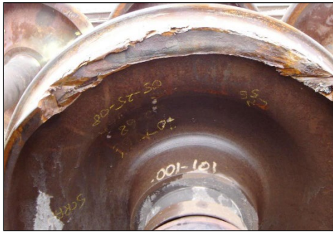
Figure 1. Vertical Split Wheel Rim
