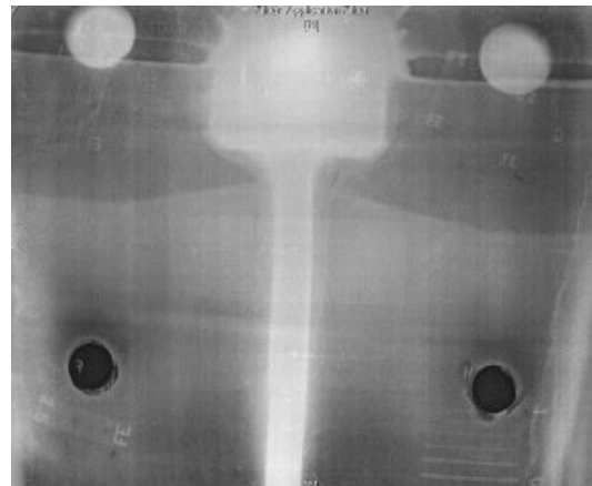
Figure 2: Radiograph of a Bolster with Minimal Defects
