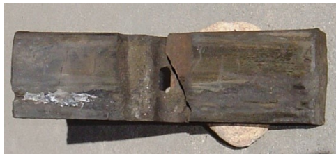
Figure 2. Composition Brake Shoe with Embedded Pickup Metal
