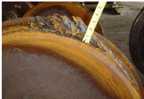
Figure 1. Wheel with TBU Extending 3 in. Radially from the Tread Surface
