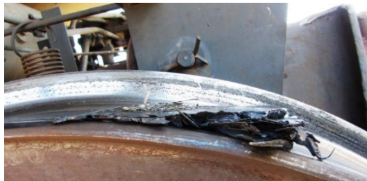
Figure 1. Wheel with TBU Extending 1 inch Radially from the Tread Surface as a Result of a Wheel Slide Test
