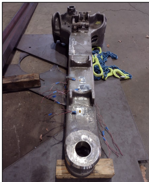
Figure 49. Test Coupler Underside - Post Test
