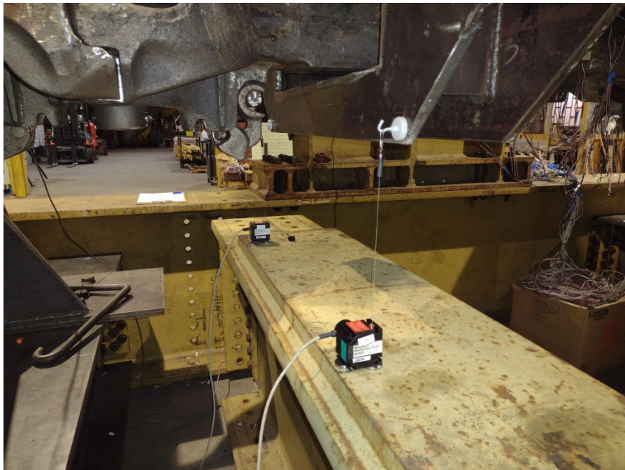
Figure B 2. Example Displacement Transducer Application
