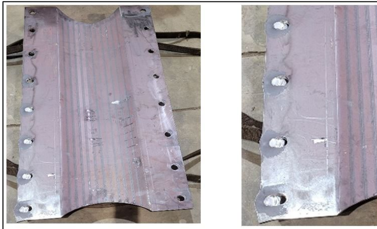
Figure 45. Hole Elongation on Retainer Plate
