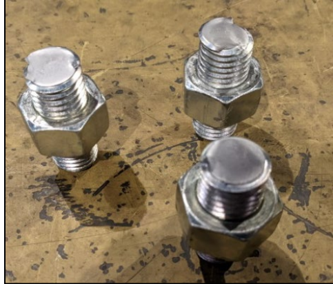
Figure 44. Shear Failure of Bolts
