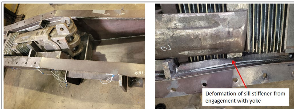
Figure 46. Post Test After Disassembly – View 1
