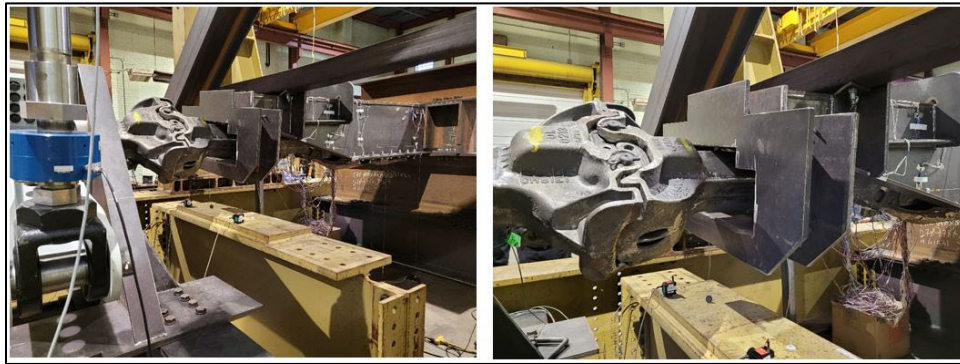
Figure 48. Rotation of Couplers – Post Test
