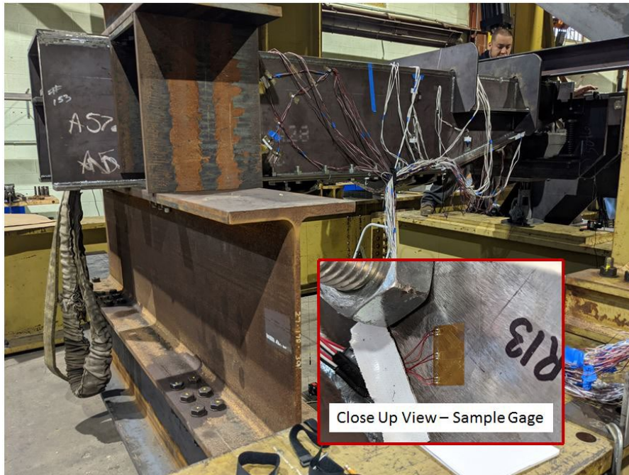
Figure B 1. Example Strain Gauge Application
