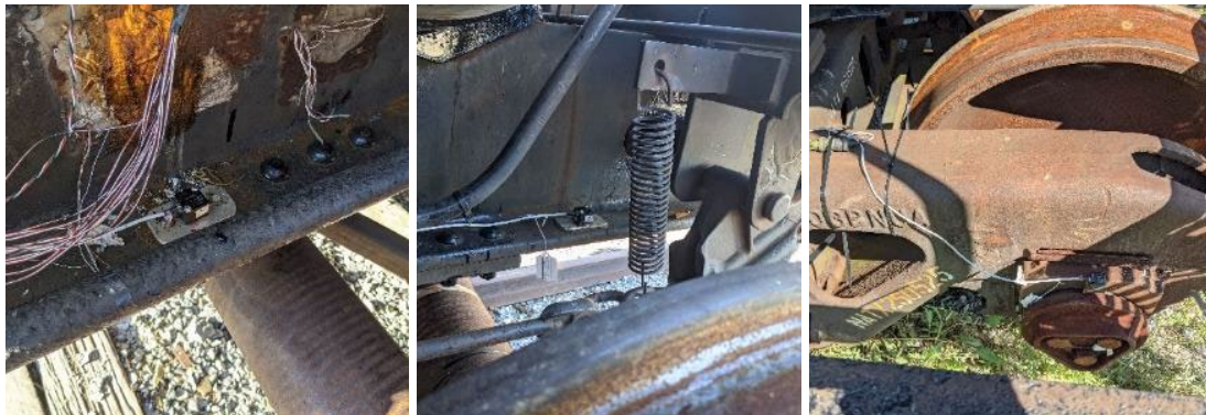
Figure 14. Accelerometers Mounted on the Stub Sills and Axle (Stub Sill A-End on Left, Stub Sill B-End in Center, Axle on Right)
