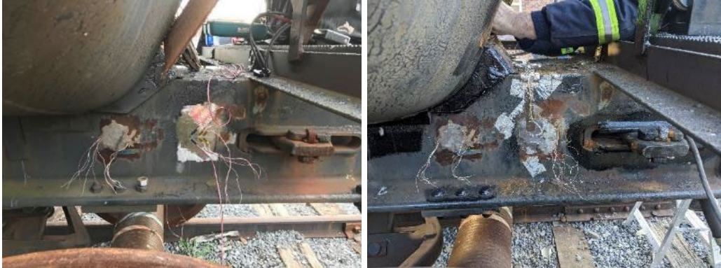
Figure 7. Strain Gages Installed on the Stub Sill for Measuring Vertical Coupler Force (Old on Left, New on Right)
