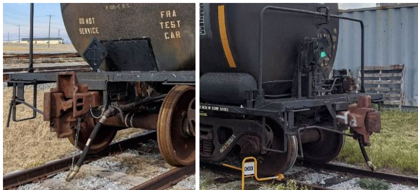
Figure 6. Instrumented Couplers for Measuring Longitudinal Coupler Forces (A-End on Left, B-End on Right)
