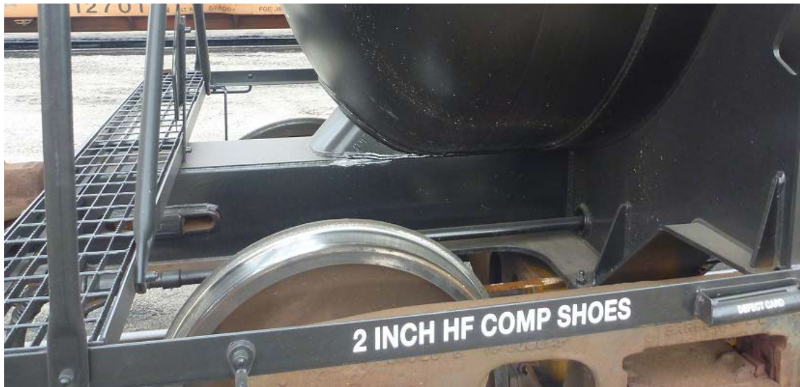
Figure 4. Detail View of the Stub Sill and Head Brace Attached to the Tank of the Instrumented Tank Car
