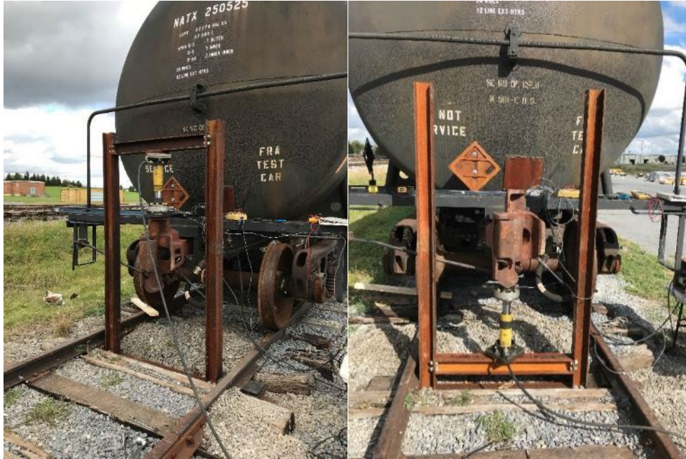
Figure 17. Vertical Coupler Force Calibration Setup (Downward Force on Left, Upward Force on Right)
