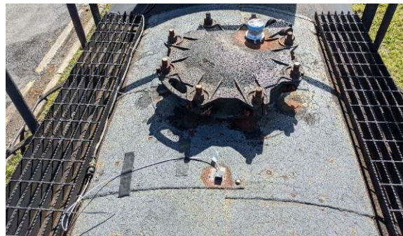
Figure 13. Tri-Axial Accelerometer Mounted on Top of the Carbody
