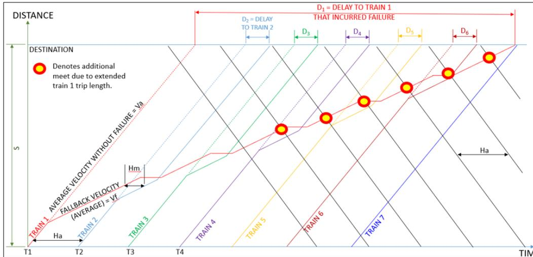
**Figure 3. Train delays in the network due to a train operating with PTC onboard cutout**
