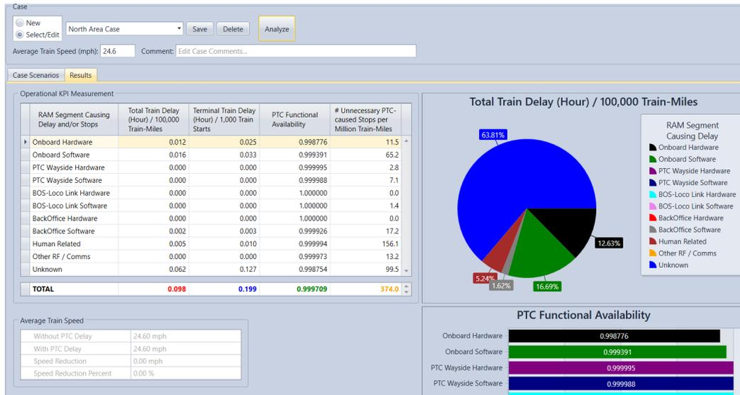
**Figure 17. Example of partial results of RAM KPI calculation for individual PTCIEs**
