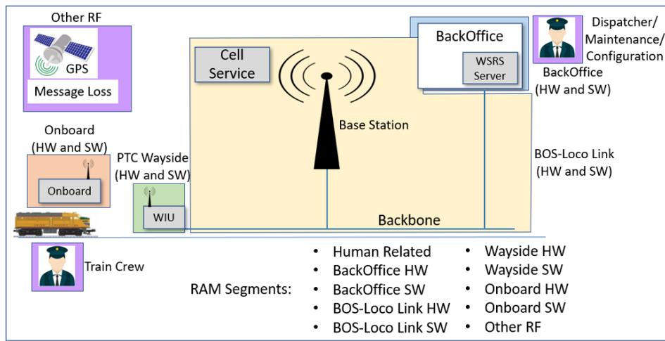
**Figure 1. Illustration of PTC RAM segments**
