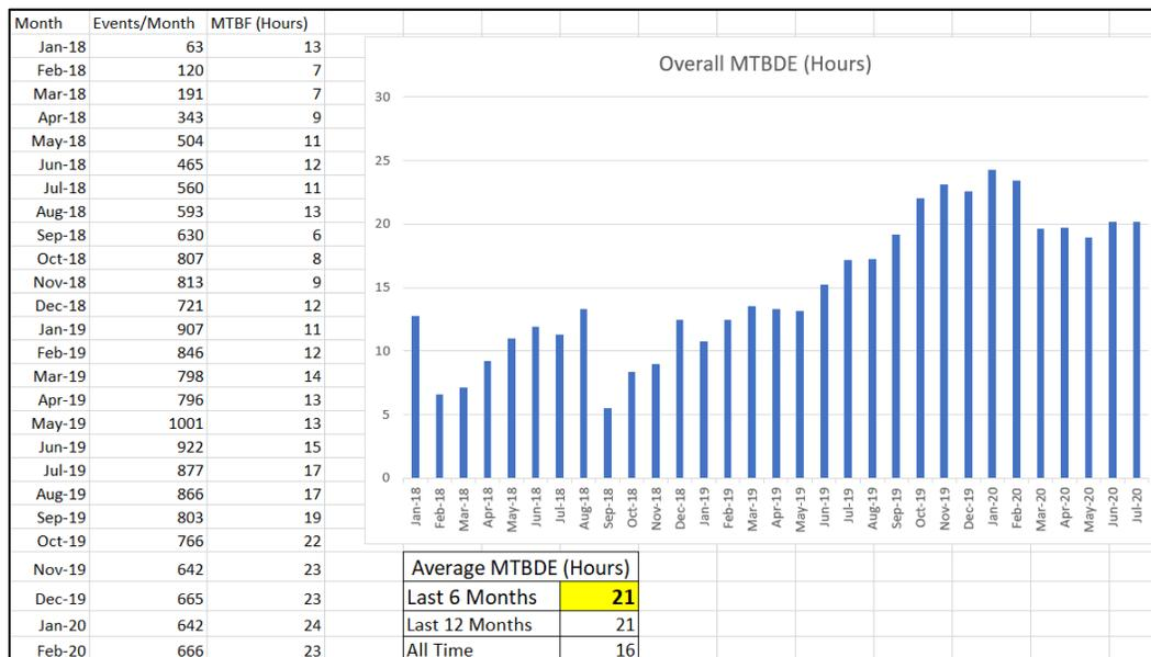
**Figure 63. Illustration of MTBDE quantification for Enroute PTCIEs**
