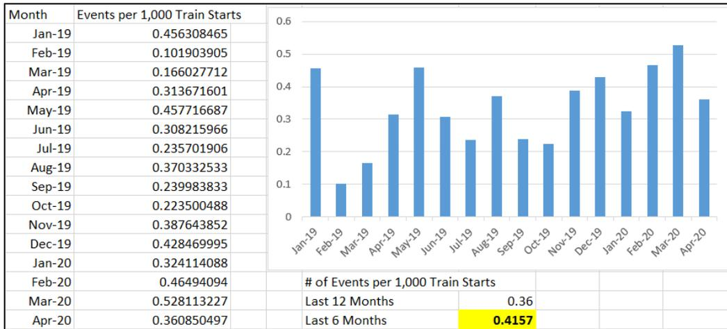
**Figure 64. Illustration of quantification of frequency of events for Terminal PTCIEs**
