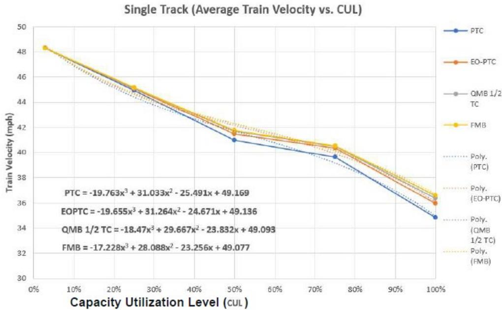
**Figure 4. Example of performance equations for signaled single track scenario**
