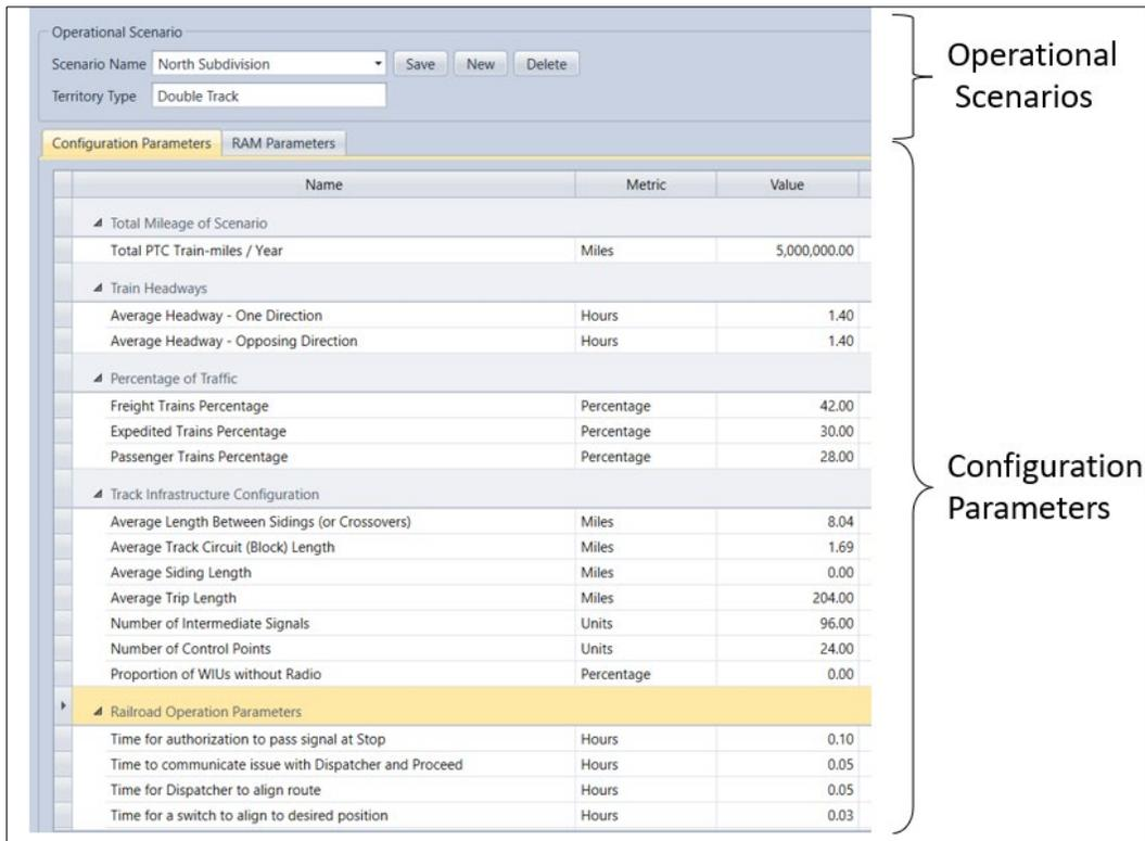
**Figure 9. Example of partial railroad configuration parameters in OPRAM**
