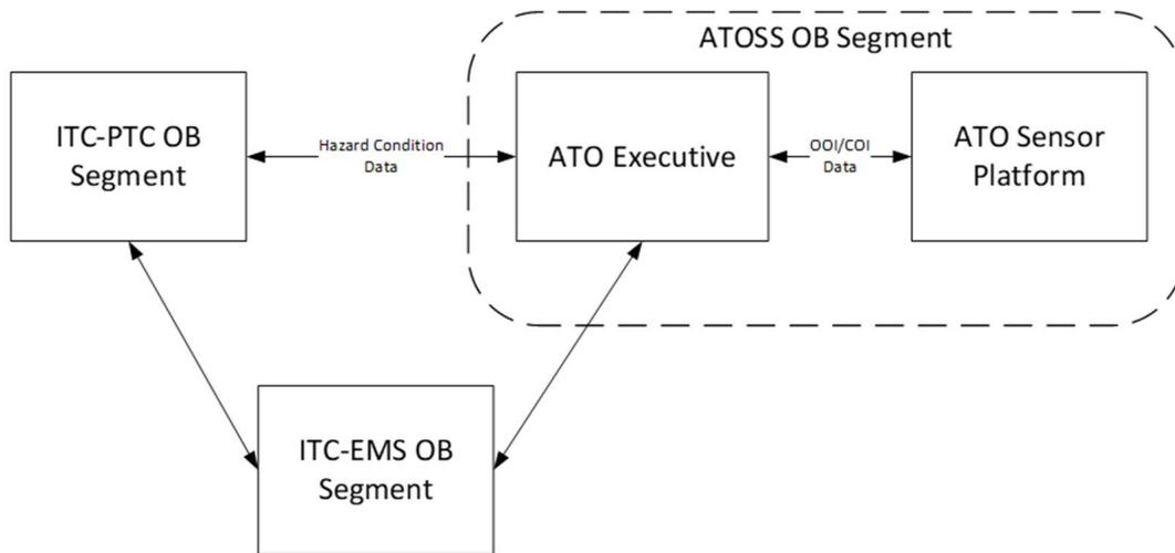
**Figure 2. ATOSS OB Segment Subsystems/Components**
