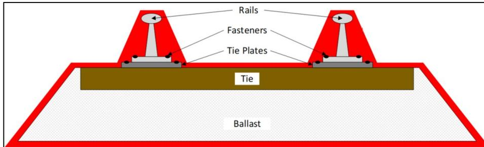
**Figure 4. Track and Road Structure**
