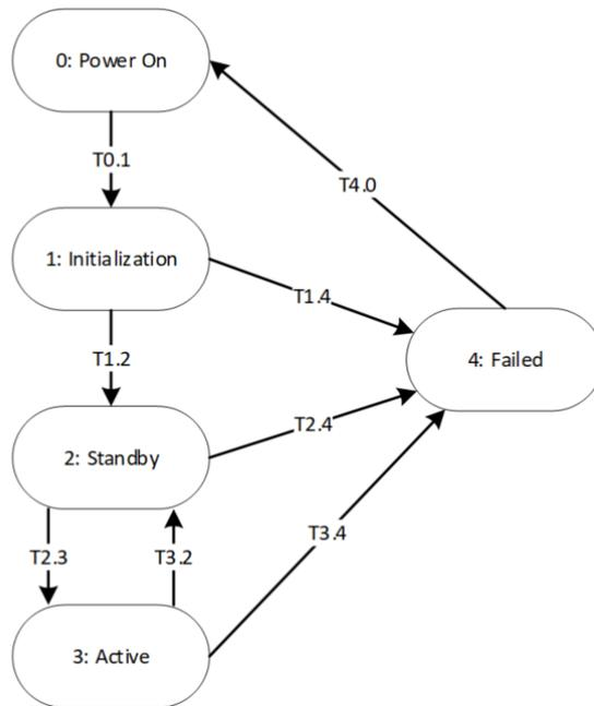
**Figure A3. SP System States Diagram**
