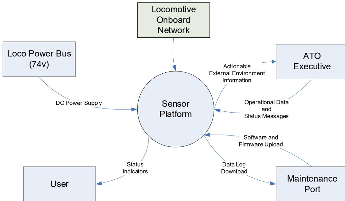
Figure A12. SP Interface Diagram
