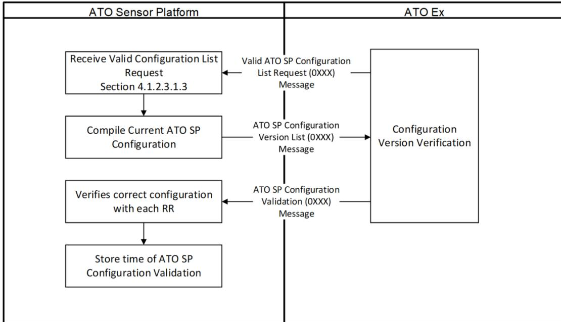
**Figure A7. SP Configuration Verification Process Diagram**
