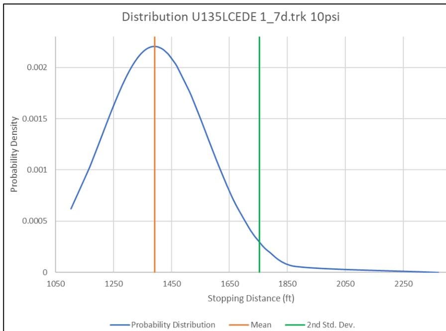
**Figure 5. Stopping Distance Distribution for Monte Carlo Simulation**
