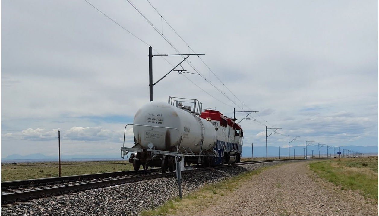
Figure 10. Train Consist Used for Wet Track Preparation
