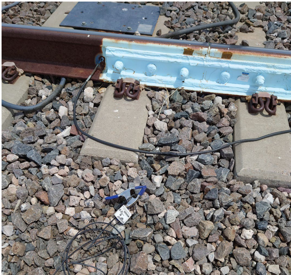
Figure 12. Broken Rail Trap During Normal Test Scenarios
