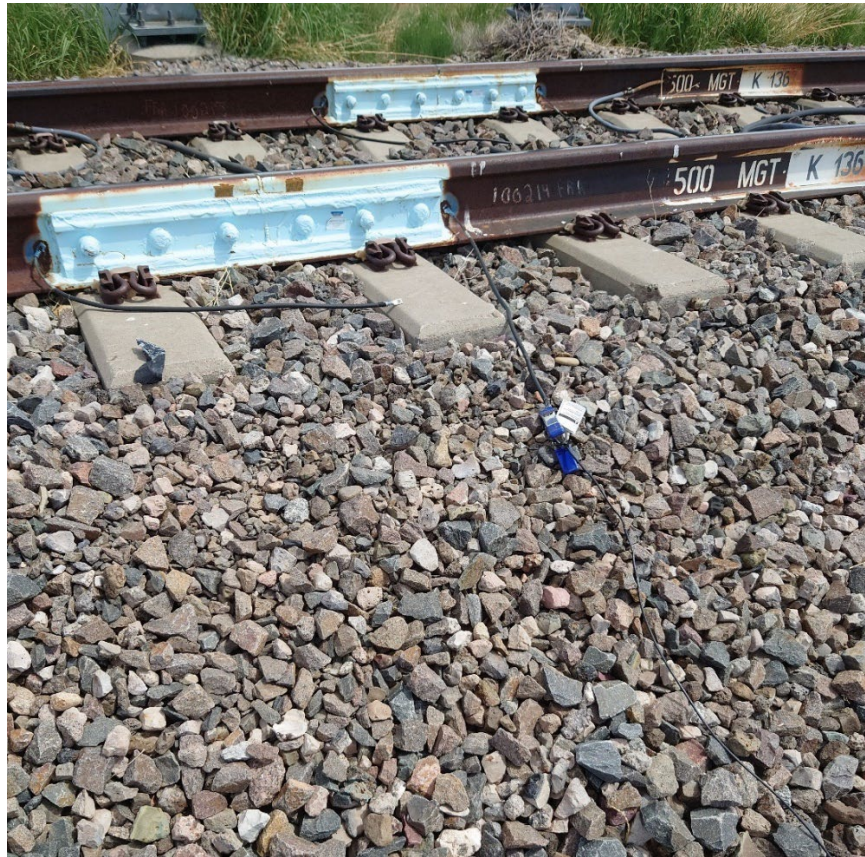
Figure 14. Clamp Mechanism for Broken Rail Test Scenarios (Disconnected)
