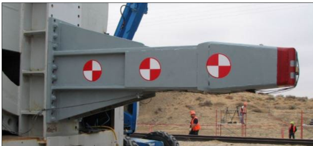
Figure 8. Ram Arm with 12 by 12-inch Indenter
