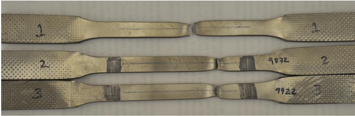
Figure 3: 295 K Specimens displaying the minor deformation at the shoulders
