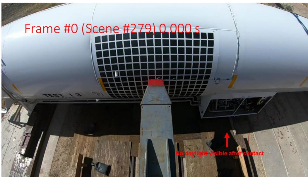
Figure 43. First Frame Showing Contact Between Impactor and Outer Tank
