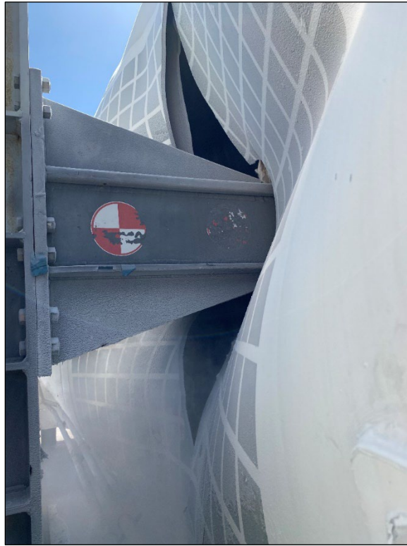
Figure 17. Ram Arm Embedded in Tank Car After Conclusion of Test
