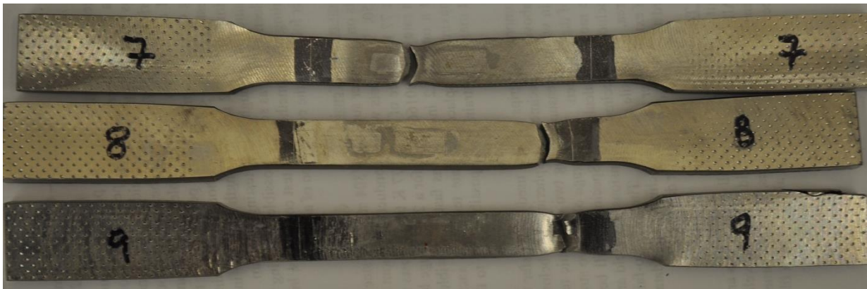
Figure 3: T304 77 K Rapid Rate Failures
