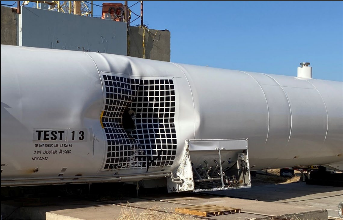
Figure 20. Tank Car after Separating from the Ram Car (impact side)
