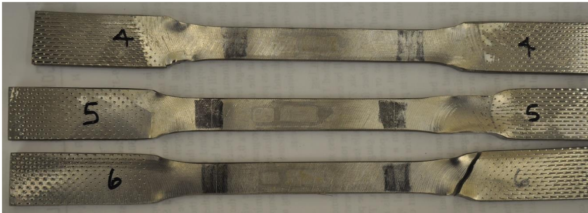
Figure 4: 77 K standard load rate specimens
