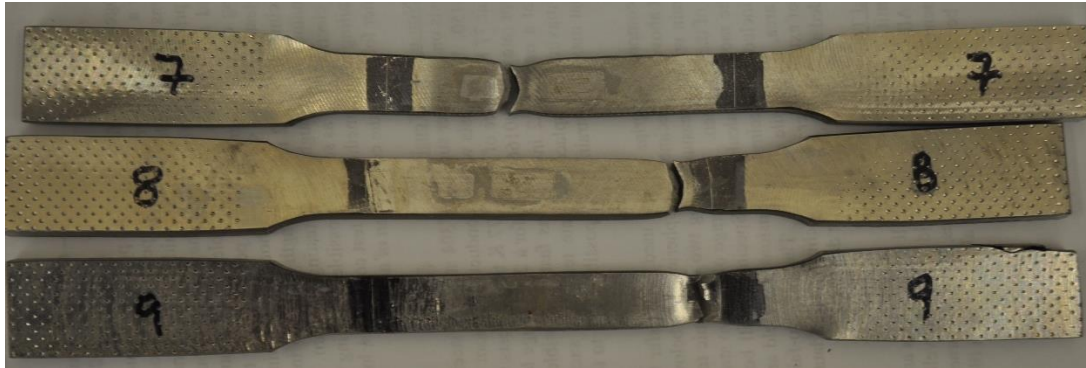
Figure 5: 77 K Rapid Rate specimens
