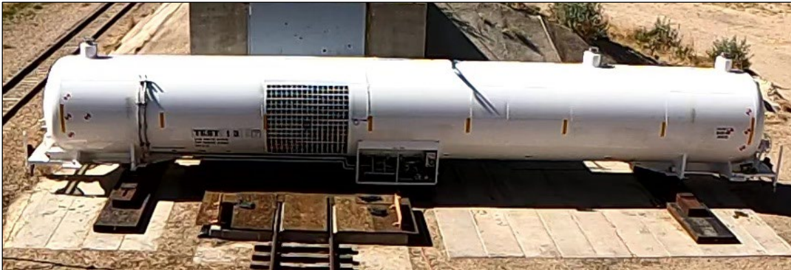
Figure 1. DOT-113 Tank Car Mounted on Support Skids
