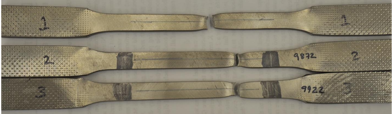
Figure 1: T304 295K Failures
