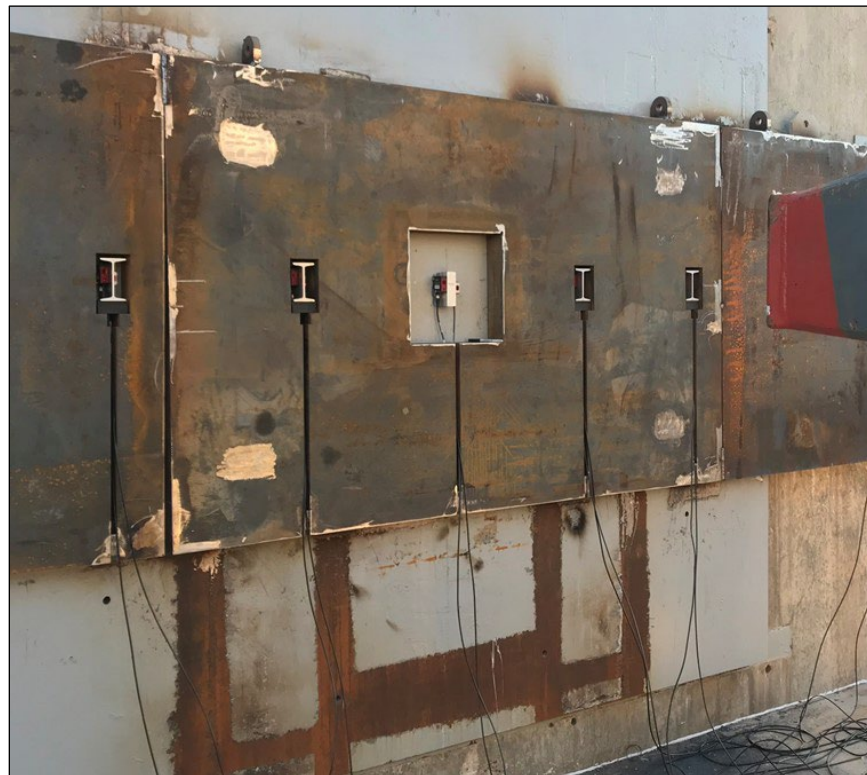
Figure 14. Lasers Displacement Transducers on Crash Wall
