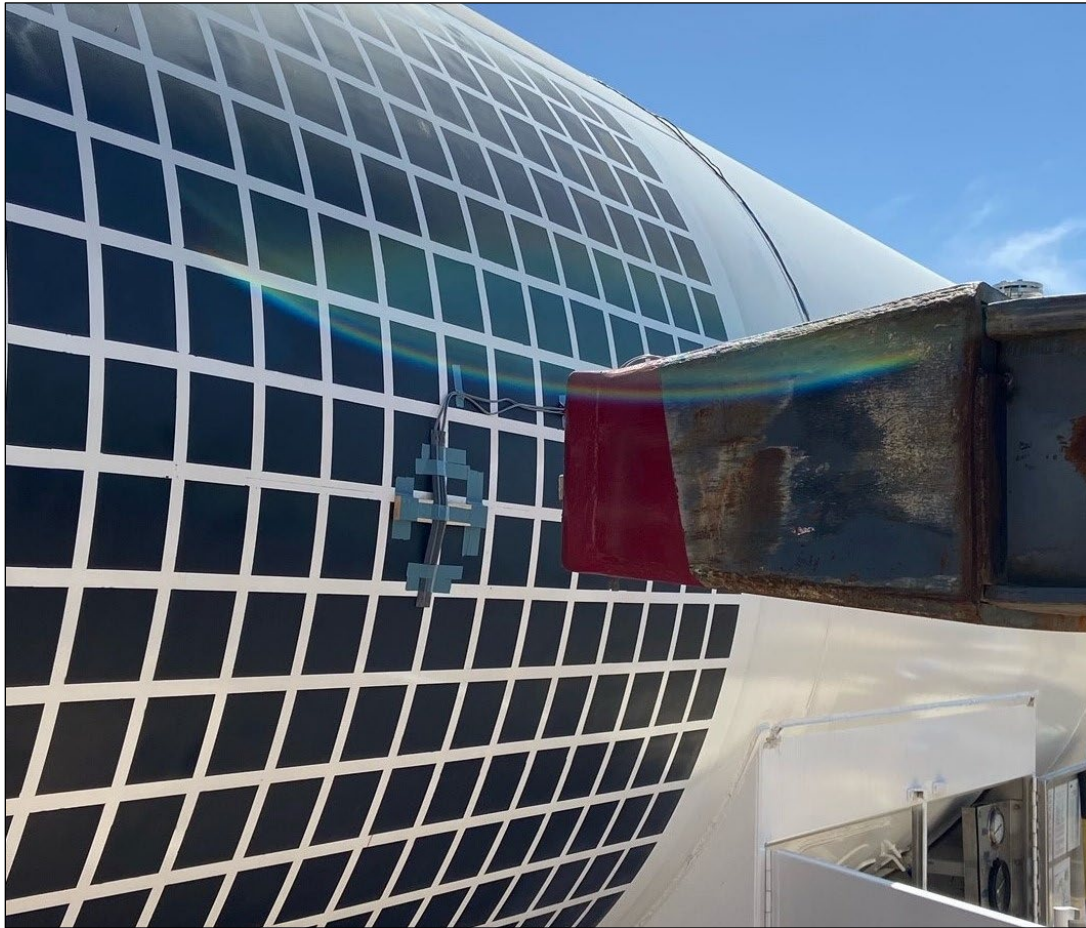
Figure 9. Ram Arm with 12 by 12-inch Indenter Aligned with the Impact Zone on the Tank Car
