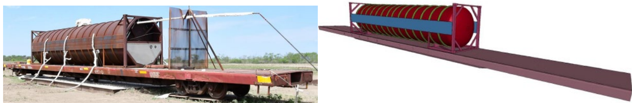
Figure 3. Physical and FE model of UN-T75 tank positioned on flatbed railcar
