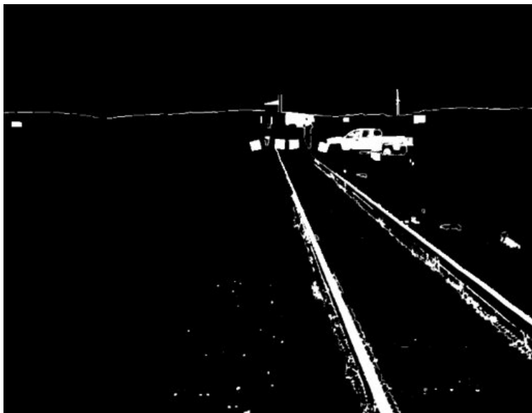
Figure 11. Binary image of the GrabCut output in Figure 9 for the fine-grained method of saliency
