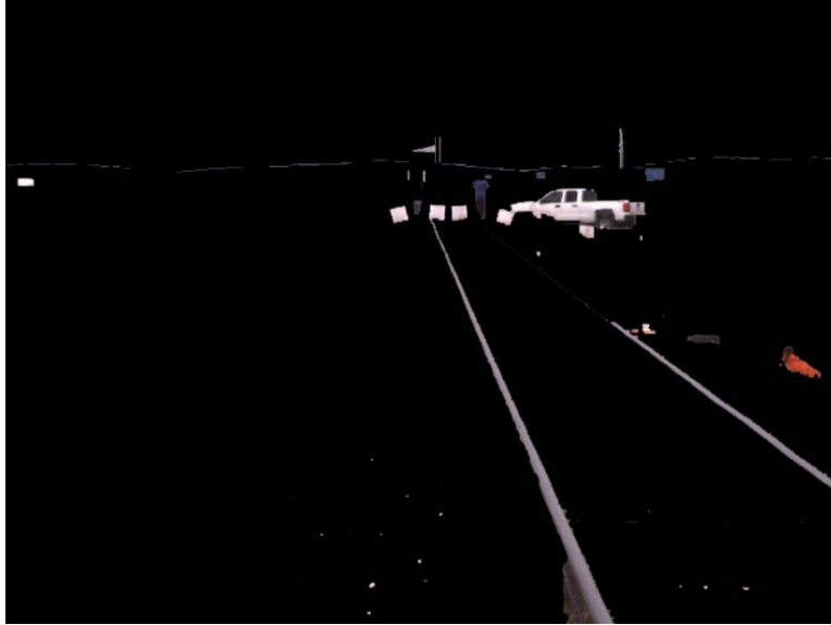
Figure 8. Foreground extracted from the input image in Figure 5, for the spectral method of saliency using the GrabCut algorithm
