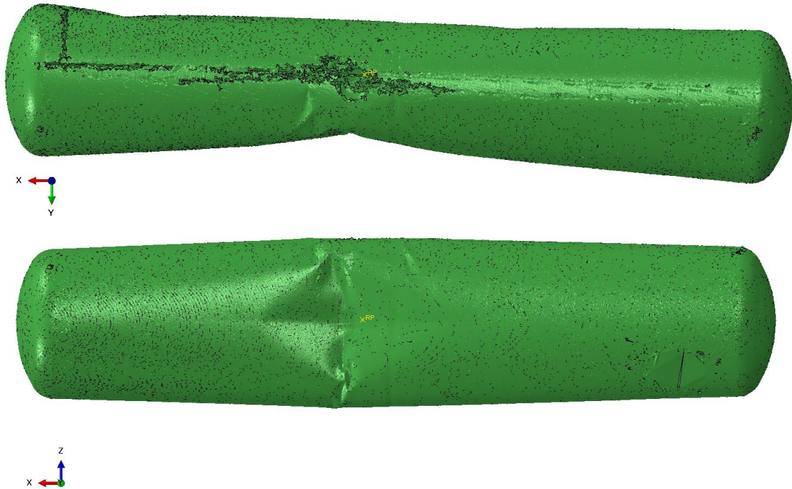
Figure E5. Post-test 12 LiDAR Scan of Inner Tank
