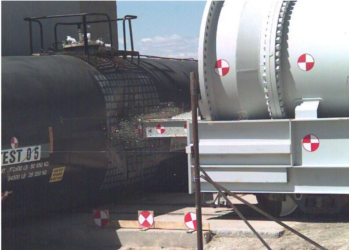
Figure 9. Deformed Tank Just Prior to Puncture (12 x 12-inch Indenter) [30]
