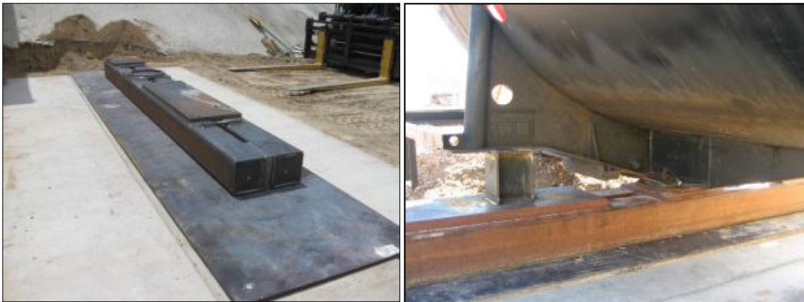
Figure 8. Tank Support Skid System [30]
