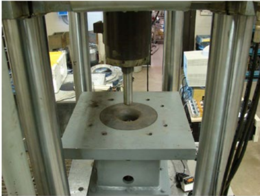
Figure 73. Punch Test and Comparison of Experimental and Numerical Results
