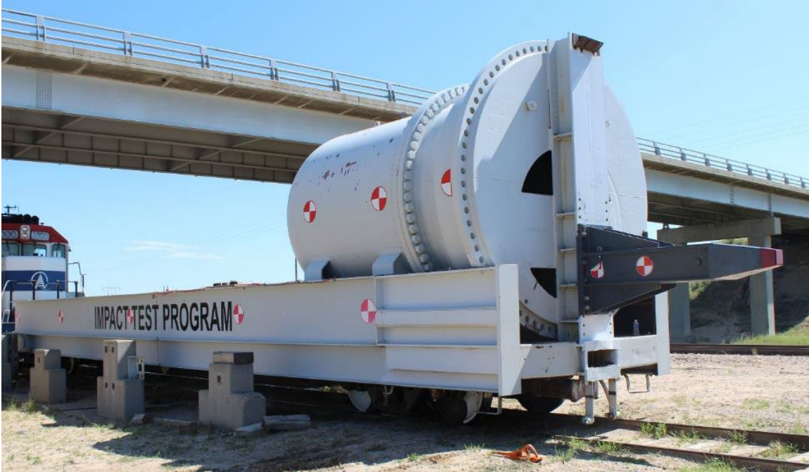
Figure 7. Photograph of a Ram Car and Head Fitted with 6 x 6-inch Indenter [30]
