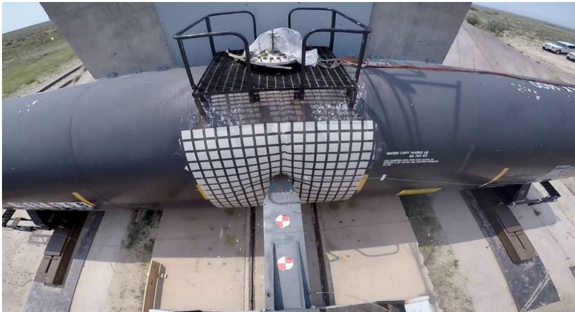
Figure 10. Deformed Tank Just Prior to Puncture (6 x 6-inch Indenter) [30]
