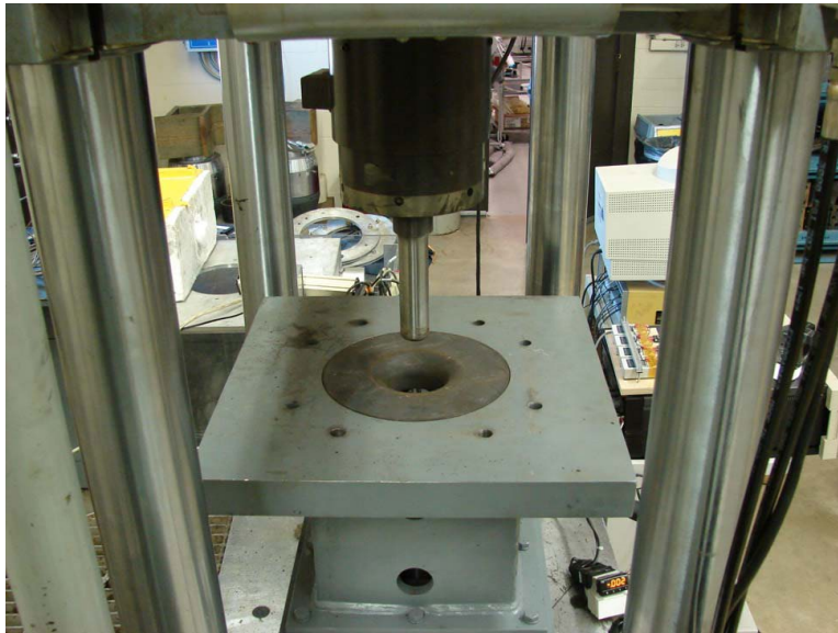
Figure 42. Simulation of the punch test on the thin TC128B plate material.
