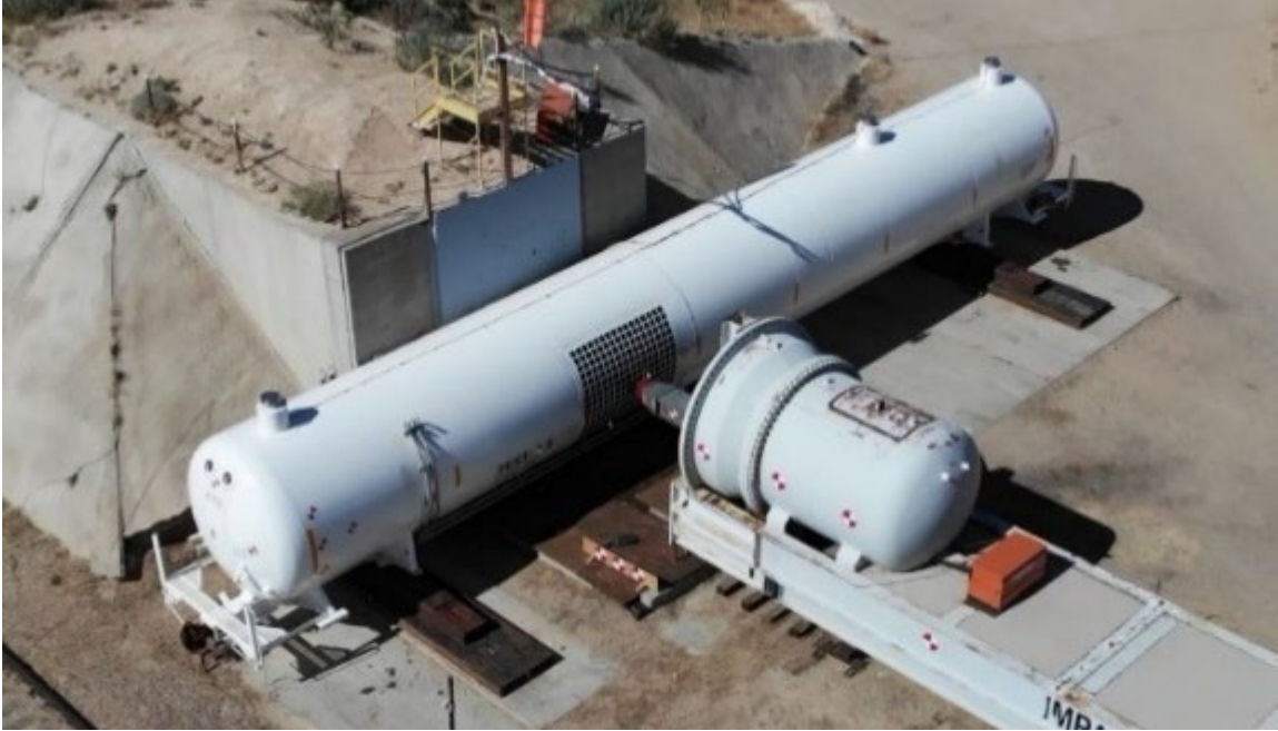
Figure 232. Pre-impact configuration of the DOT-113 tank car and ram for Test 13 (FRA, 2022).
