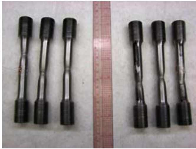
Figure 34. Necking behavior observed in the TC128B round bar specimens.
