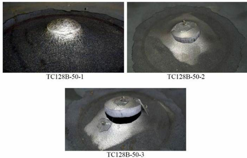
Figure 43. Punch test failure mode for the thin TC128B plate material.
