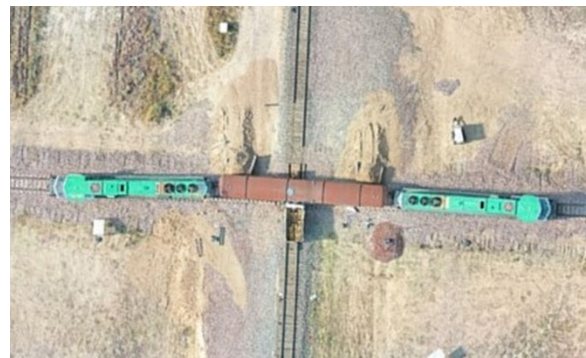
Figure 2. Orthomosaic of highway-rail grade crossing impact test
