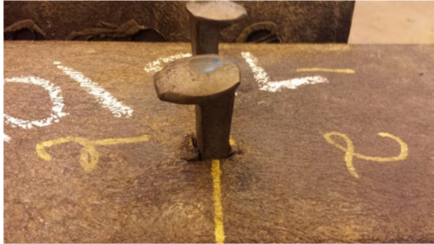
Figure 6. Mushrooming of composite material after driving a spike in the lab
