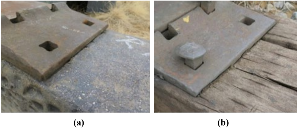
Figure 20. Plate cutting at the high rail of (a) an EPC tie after 1,690 MGT and (b) a control hardwood tie after 970 MGT, both installed in a six-degree curve at FAST
