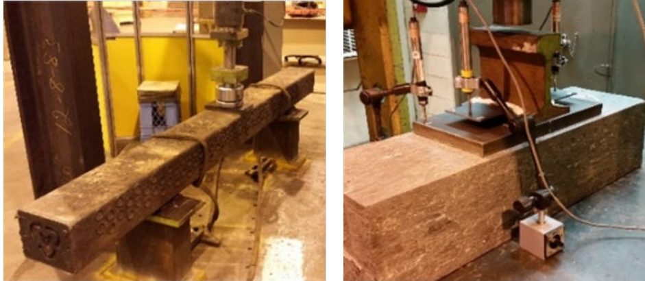
Figure 24. Tie center bending test (left) and plate compression test (right) used to tune model parameters
