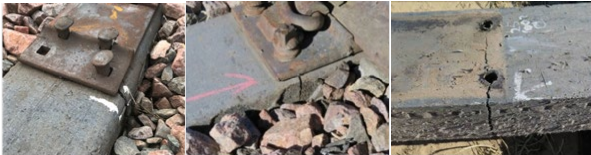
Figure 17. Spike-hole failure modes observed in EPC tie test zones
