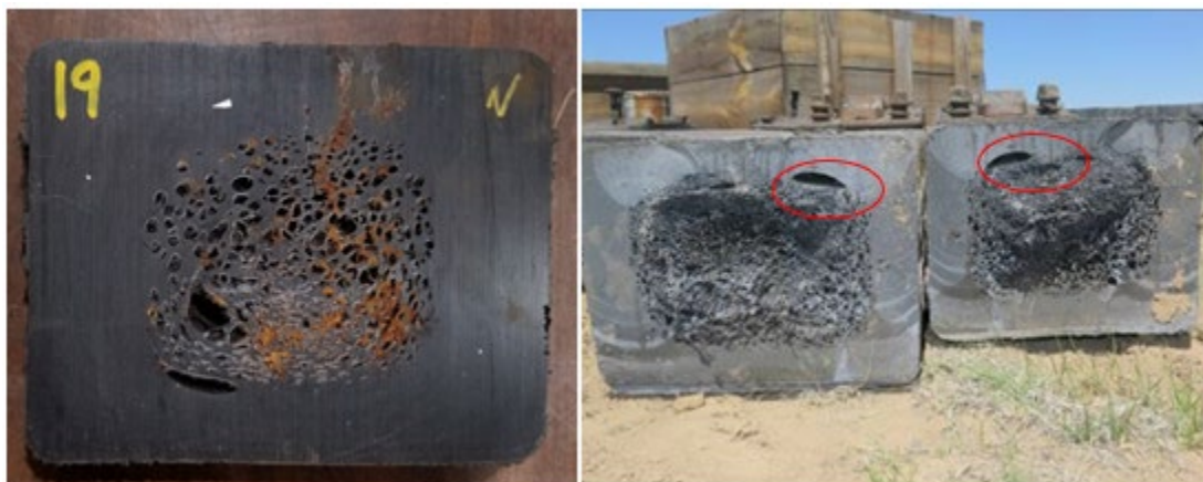
Figure 39. Internal condition of laboratory tested tie vs. in-track failed tie
