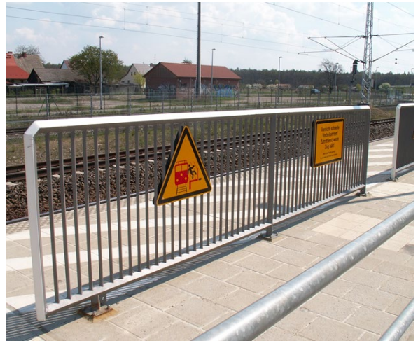
Figure 3-8. Examples of platform screen doors and barriers. Top: full-height doors in China [11]. Bottom-left: part-height solid barriers in Japan [29]; Bottom-right: barrier fences in Germany [13]
