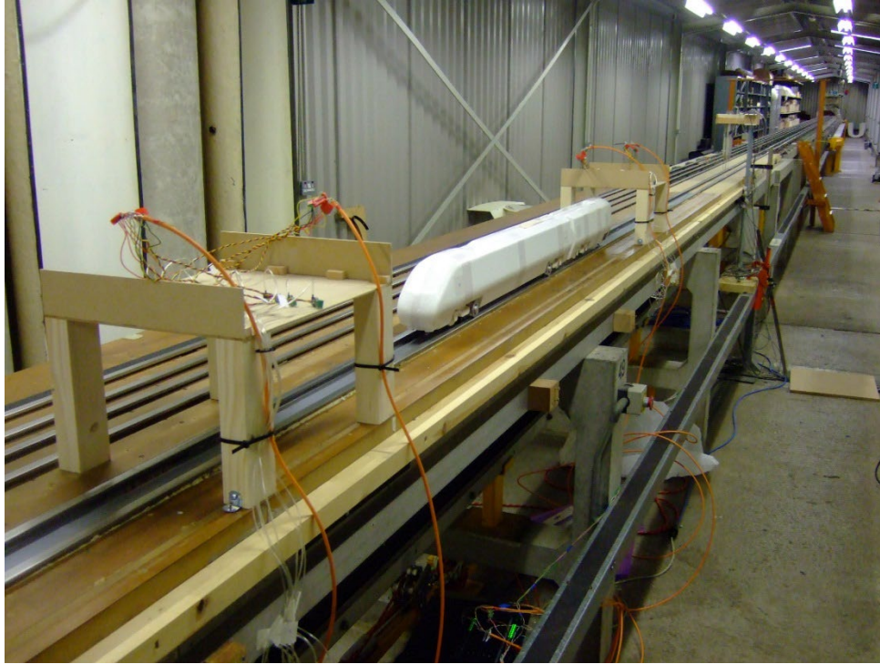
Figure 2-6. The “TRAIN rig” reduced-scale moving model testing facility in Derby, England, set up to measure pressure on a short overhead canopy; photo courtesy of Birmingham Centre for Railway Research and Education
