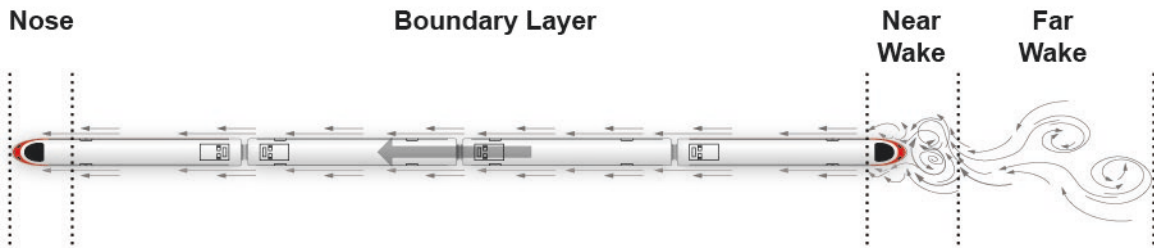
Figure 3-1. Illustration of the airflow around a train, with the regions of the slipstream identified
