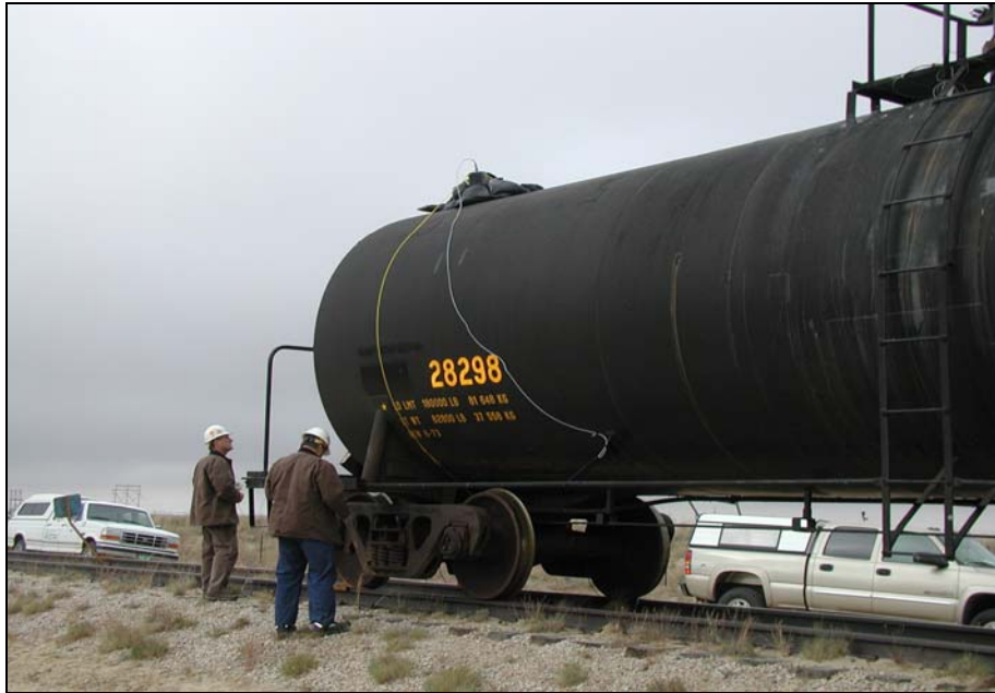
Figure 12. Preparation of Vent Charge for Test 1, A-End of Car
