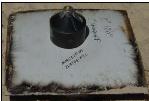
Figure 10. 10-Inch x 120-Degree Shape Charge on Test Sample
