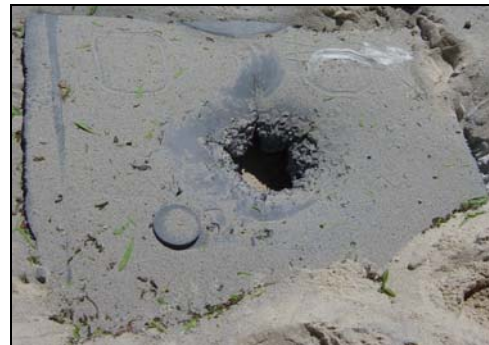
Figure 11. Hole from 10-Inch x 120-Degree Shape Charge on 5/8-Inch Shell and 11-Gage Jacket
