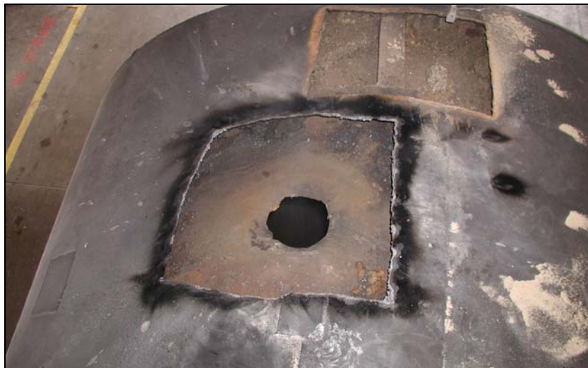
Figure 16. Vent Hole from Test 1 Using Helix-Shape Charge
