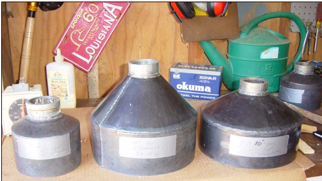
Figure 3. 6-Inch x 120-Degree, 10-Inch x 90-Degree, and 10-Inch x 120-Degree Shape Charges
