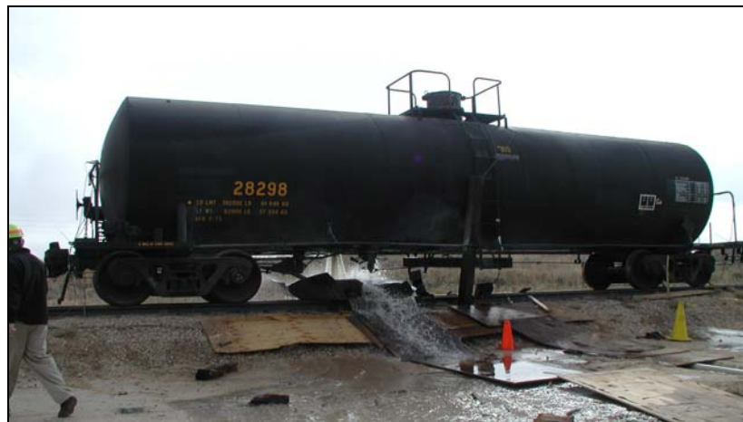
Figure 14. Water Draining After Full-Scale Vent and Drain Test 1
