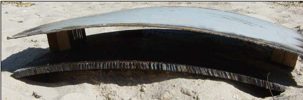
Figure 9. Typical Test Sample for Coupon Test
