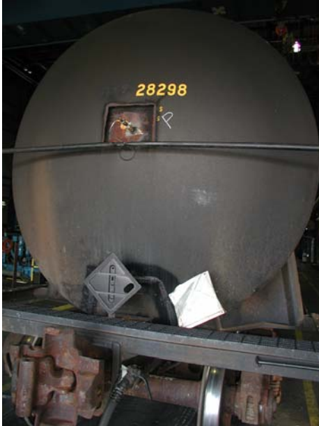
Figure 4. Pressure Transducer in A-End Tank Head
