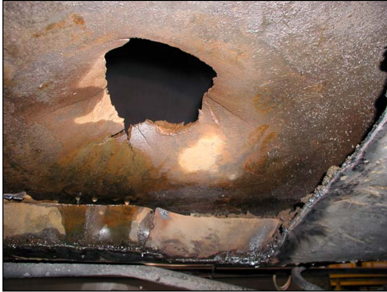
Figure 19. Drain Hole from Test 2 Using Composition B-Shape Charge
