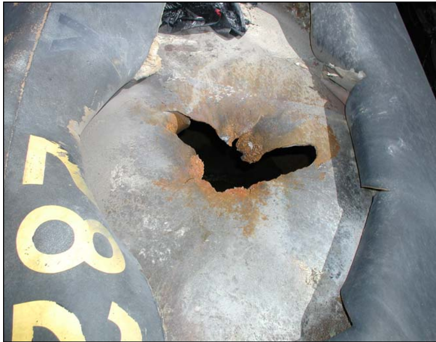
Figure 18. Vent Hole from Test 2 Using Composition B-Shape Charge
