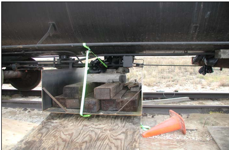
Figure 13. Drain Hole Charge for Test 1, Near the A-End of Car
