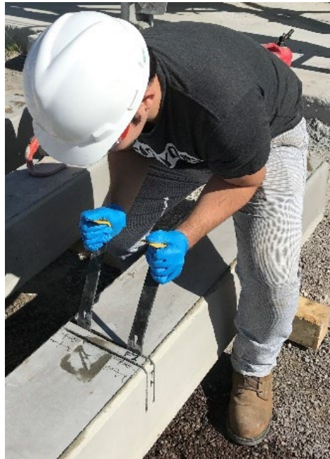
Figure 7. Sample extraction from a concrete crosstie
