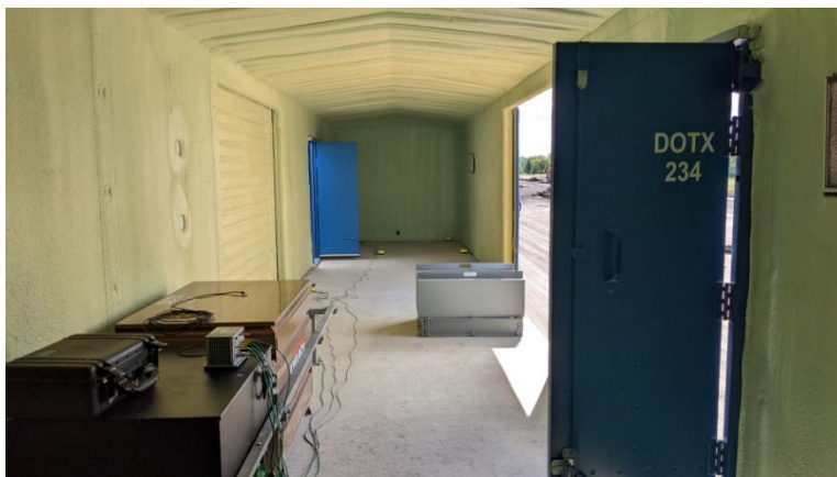
Figure 5. Inside of Instrumented Box Car DOTX 234
