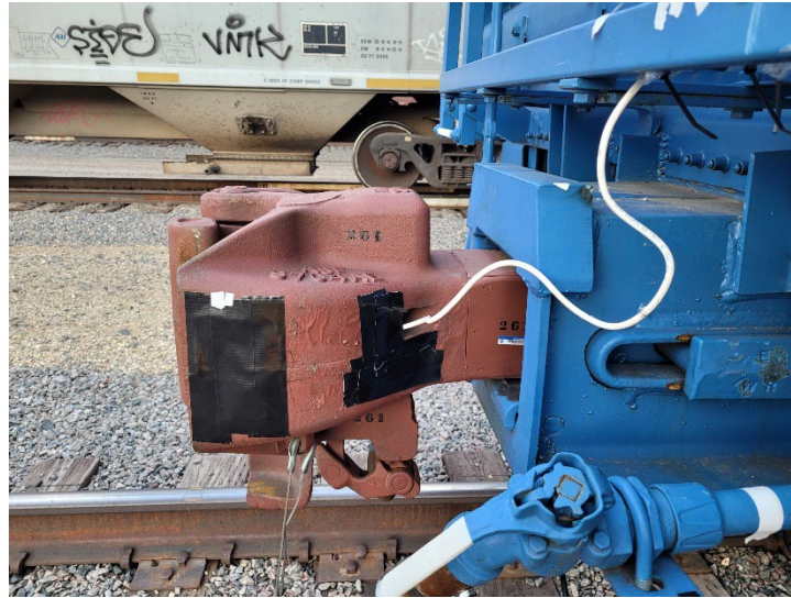
Figure 3. Instrumented Coupler Mounted on a DOTX Car
