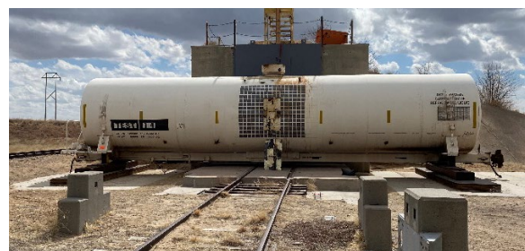
Figure 2. Post-impact DOT-105 (Jacket Removed)
