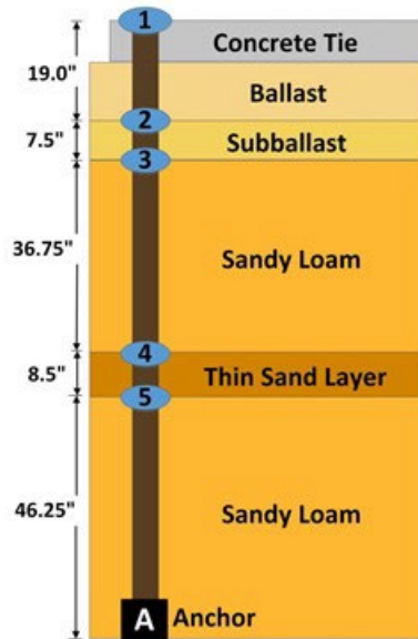
Figure 10. Subsurface profile for MDD location at Upland (15)
