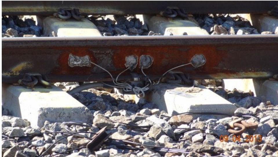
Figure 15. Two strain gages in crib area for vertical wheel load and two strain gages above the tie for tie reaction
