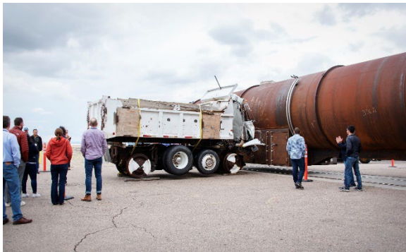
Figure 1. Decarbonization workshop tour of TTC in Pueblo, CO, showing dump truck impacts on a tank car natural gas fuel tender
