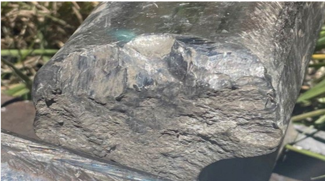
Figure 2: Batter marks on the broken rail
