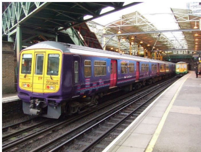
(The third rail that other trains use is visible beside the track. Creative Commons photo by Hugh Llewelyn accessed via Wikimedia Commons)
