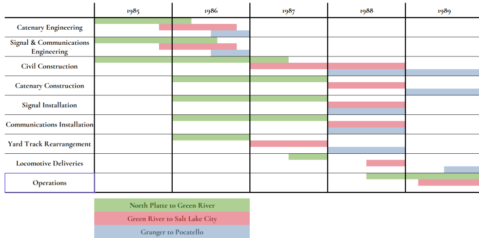
Figure 4. Planned Construction Timeline for the UP Electrification
