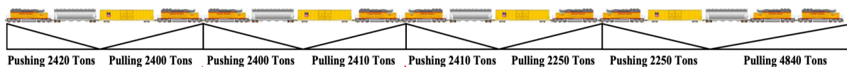
Figure 23. Example of Distributed Power Operations for a Train is Moving from Left to Right
