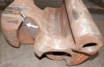
Knuckle FEA showing high stress in pulling lug (Chunduru, 2011) and knuckle failure in similar region.
