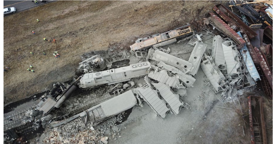
Aerial photograph of a train accident with EOT failure as a contributory cause. (NTSB)
