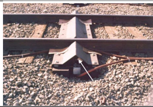
Figure 16: Impactor style DED showing location of an accelerometer on the underside of the strike plate
