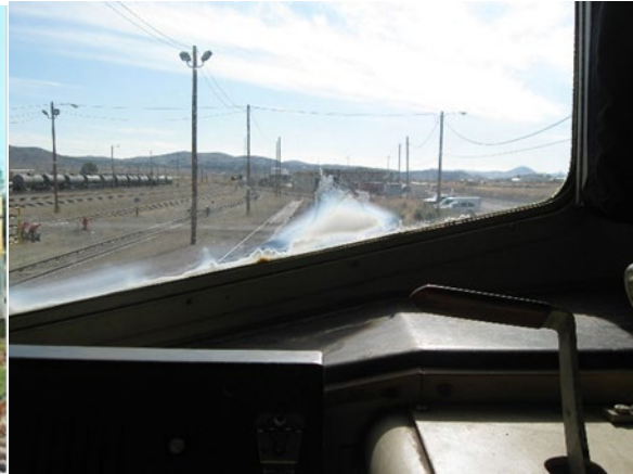
Figure 2: Locomotive with FRA-approved Type I (end facing) glazing (degraded)
