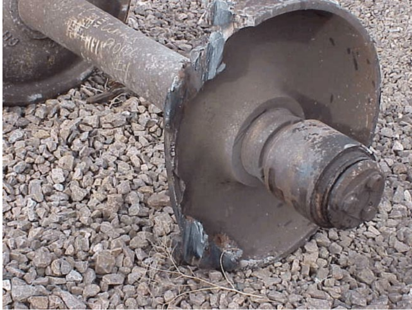
Figure 5: Split rim wheel failure
