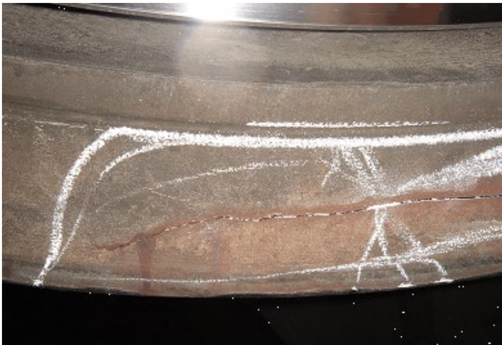
Figure 7: A crack on the side of the rim and running parallel to the tread could lead to shattered rim
