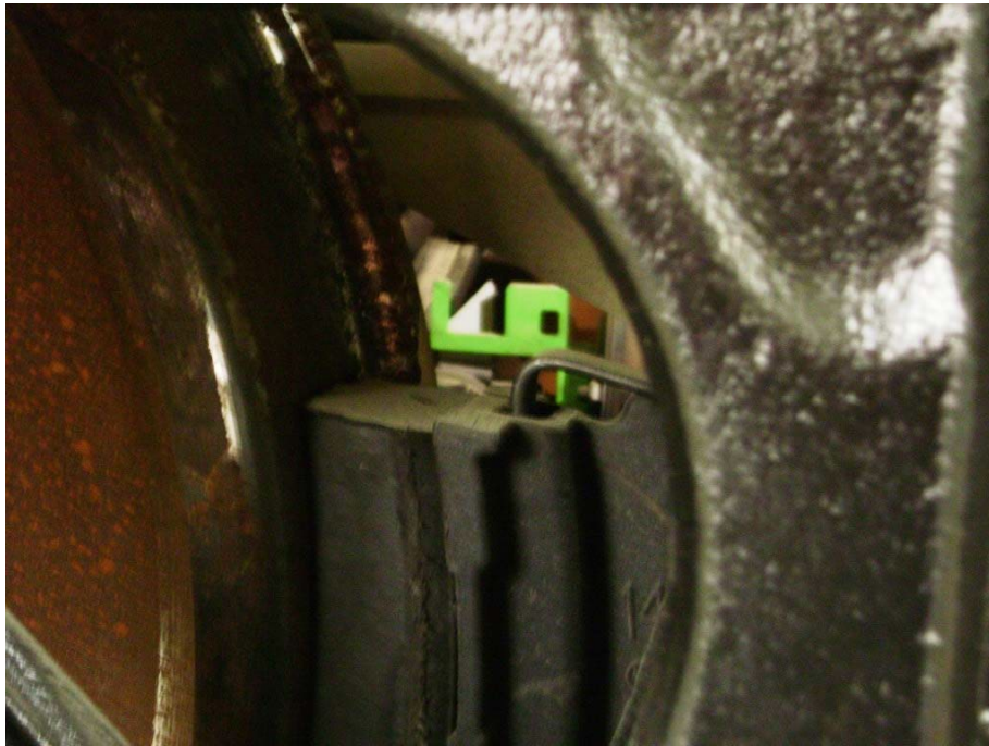
Figure 20: TMX piston travel indicator inspection
