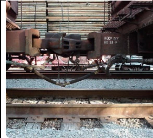
Figure 10: Air Hose State in a Train
