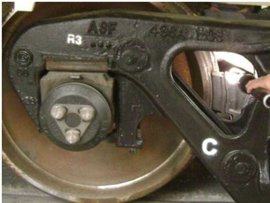
Figure 19: TMX piston travel indicator inspection
