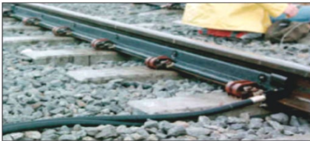
Figure: 21: Shown LIOD consists of an Angle Iron bolted to Rail at every Tie Location and anchored with Rail to Ties with Elastic Clips. The Angle Iron is instrumented on Crib Locations to measure Wheel Loads. As shown, the LIOD can be detached and anchored as needed
