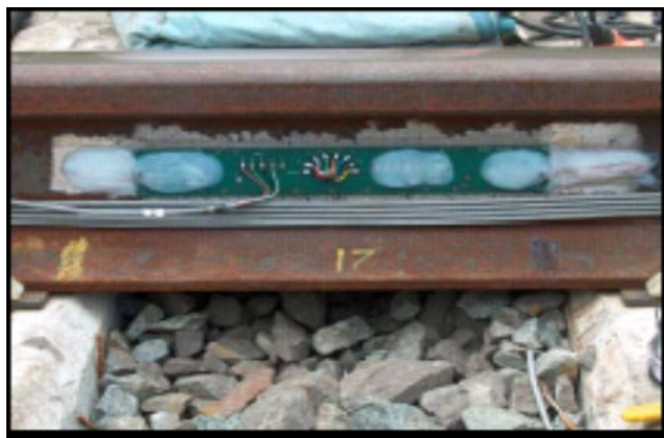
Figure 2: A Typical Strain Gage Installation on Rail Web over a Crib
