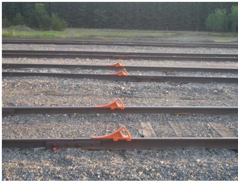
Figure 2. Skates at clearance points. Noncompliant for securement.
