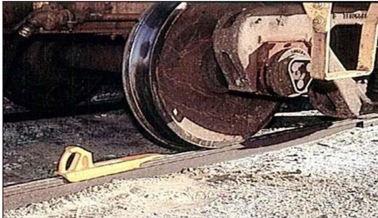
Figure 3. Skate is not engaged. Noncompliant for securement.
