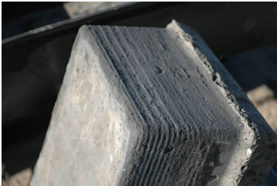
Figure A2. Tie Number 190, Showing Impressions from the Boot Ribs
