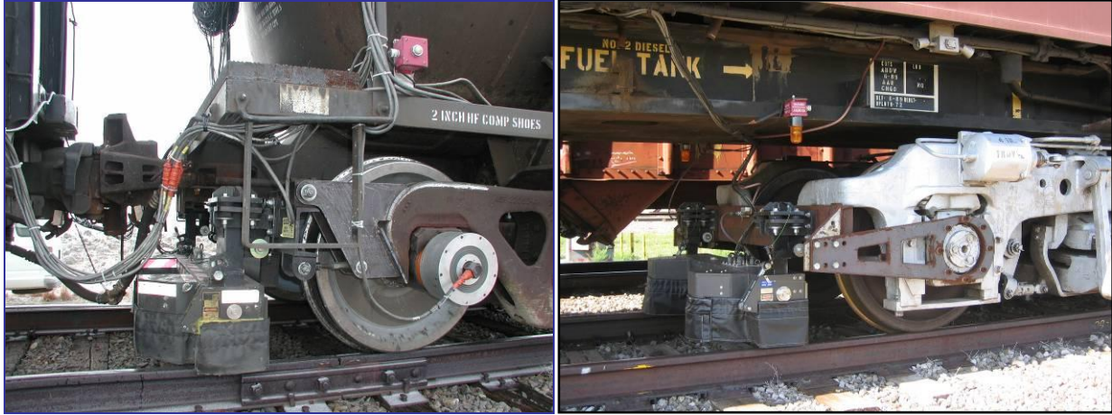
Figure 18. TTCI's Track Geometry Measurement System Attached to an Empty Tank Car (left) and TTCI's Track Loading Vehicle (right)
