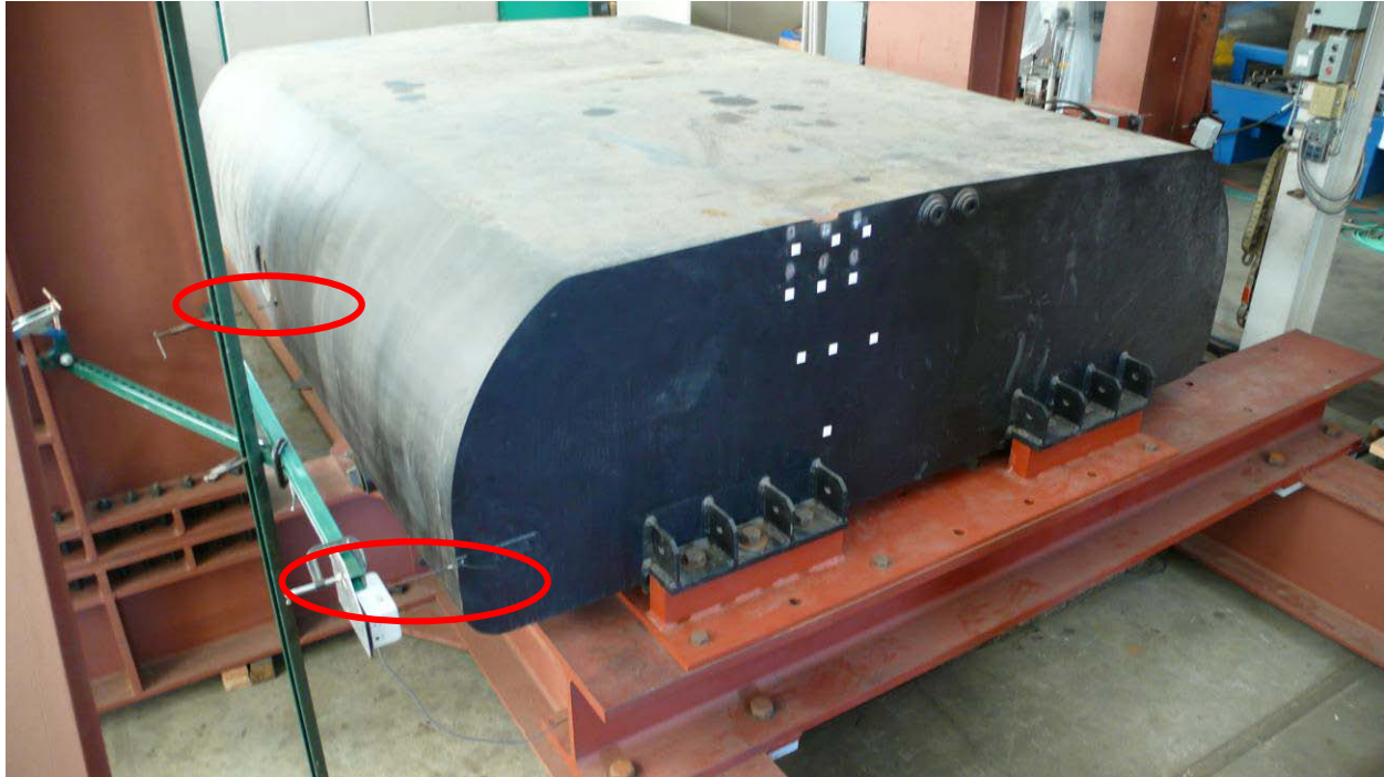
Figure 8. Two String Potentiometer Attachments to the Unloaded Sidewall of the Tank
