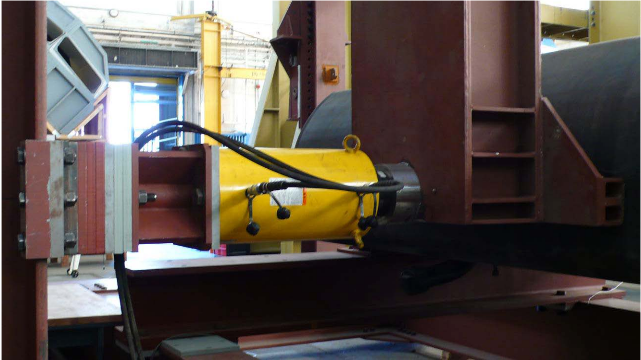
Figure 9. Configuration of Servohydraulic Actuator for Side Impact Load Application
