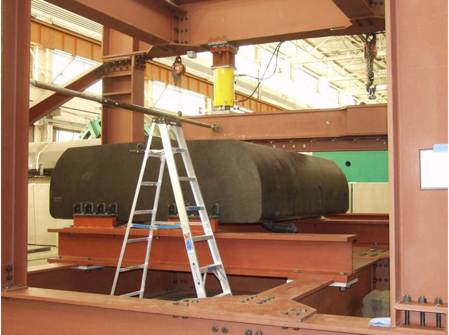
Figure 12. Test Setup with a Strut Laterally Supporting the Load Lever
