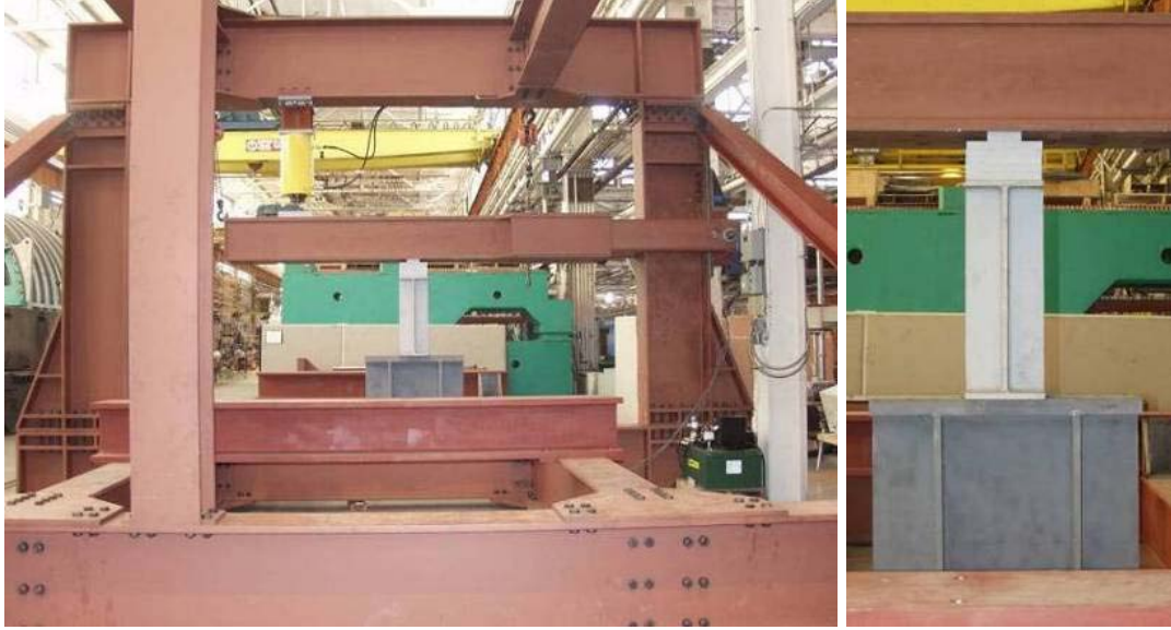
Figure 5. Fulcrum Calibration Test Setup at FMI Tank Test Facility
