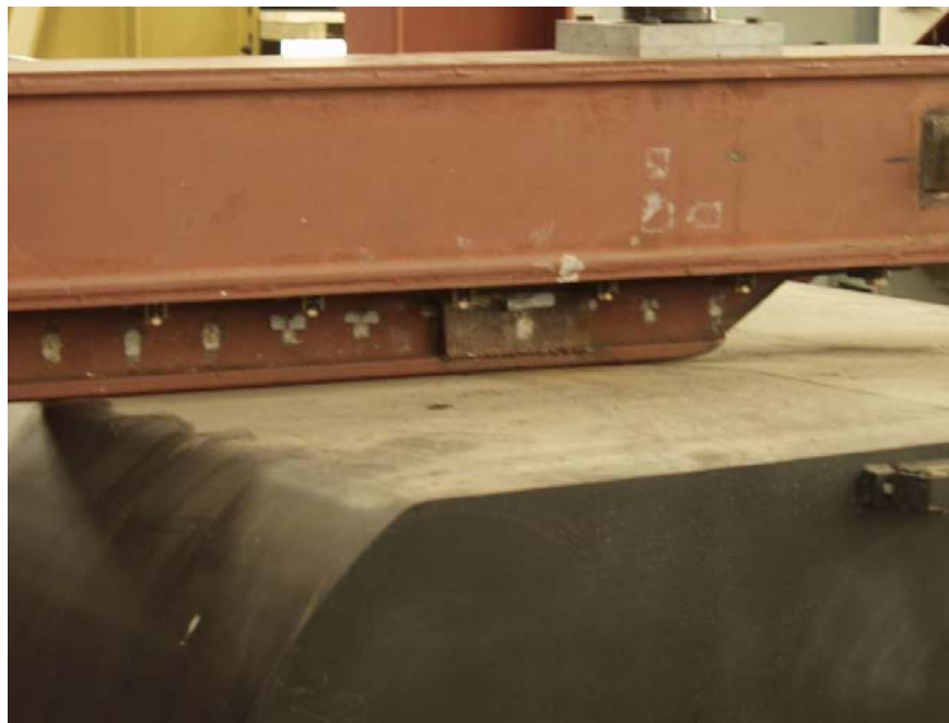
Figure 15. Undeformed Shape of Inverted Tank Bottom Wall in Contact with Rail before Test
