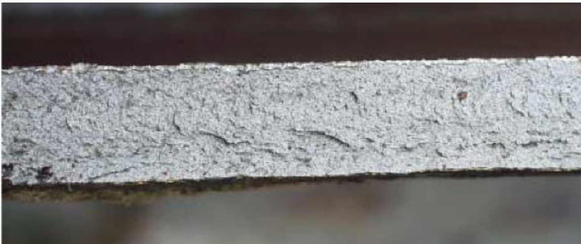
FIGURE 2.2 Brittle fracture in an anhydrous ammonia tank car that derailed near Minot, ND [1].
