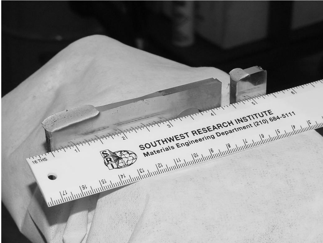
Figure 34. Typical Flat Fracture Surfaces Observed in Bend and C(T) Specimens
