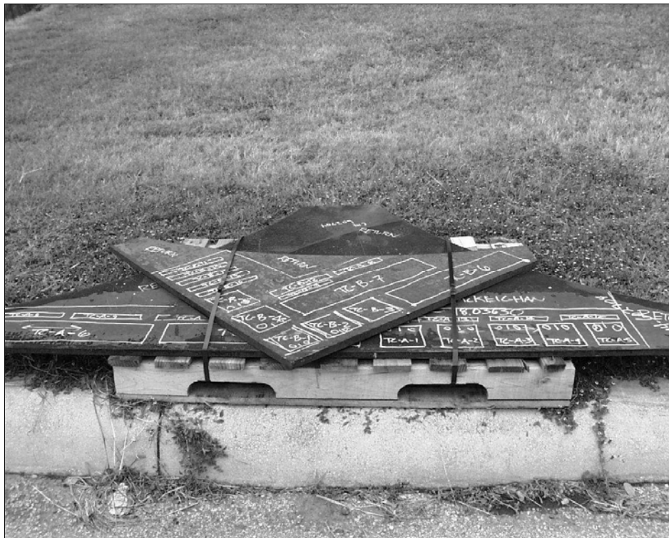
Figure 10. Plate Material Prior to Shipping to the Machine Shop for Fabrication of Specimens
