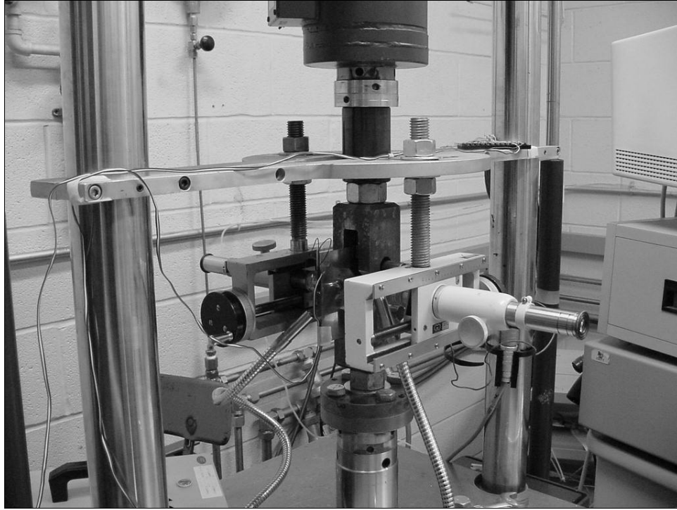
Figure 11. FCG Testing Setup for the C(T) Specimen Geometry Used in Phase A
