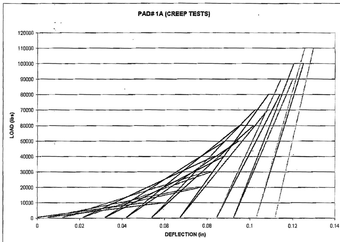
Figure 40. Typical Load-Deflection-Creep Curve for a Pad
