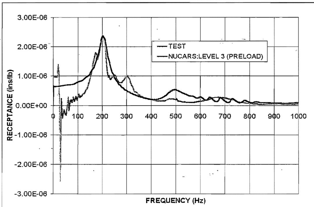
Figure 18. Test/NUCARS Model: Matching of Receptance Amplitudes
