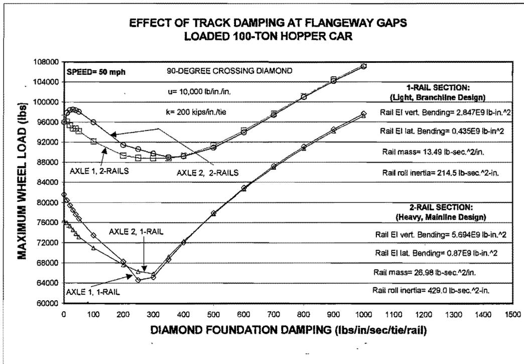
**Figure 4. Effect of Track Damping on Maximum Wheel Impact Loads:
