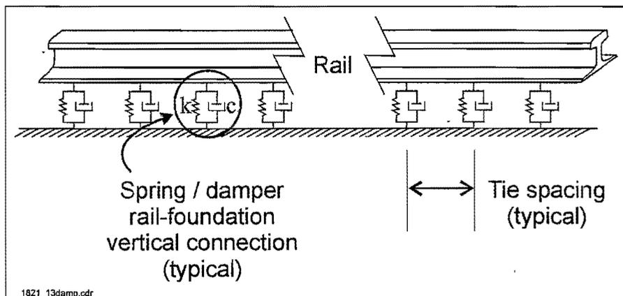
Figure 16. One-layer NUCARS Track Model for Vertical Vibrations
