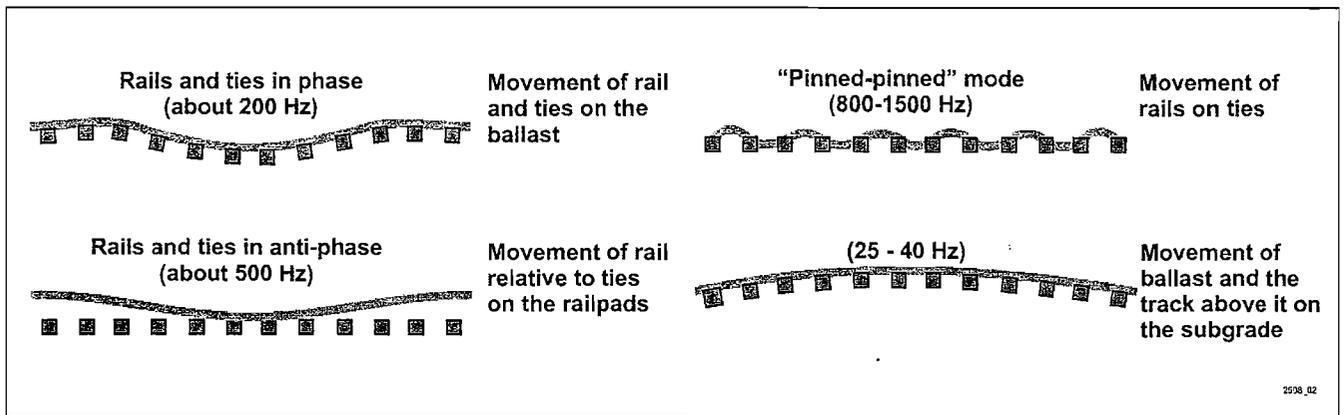
Figure 2. Typical Ballasted Track Responses
