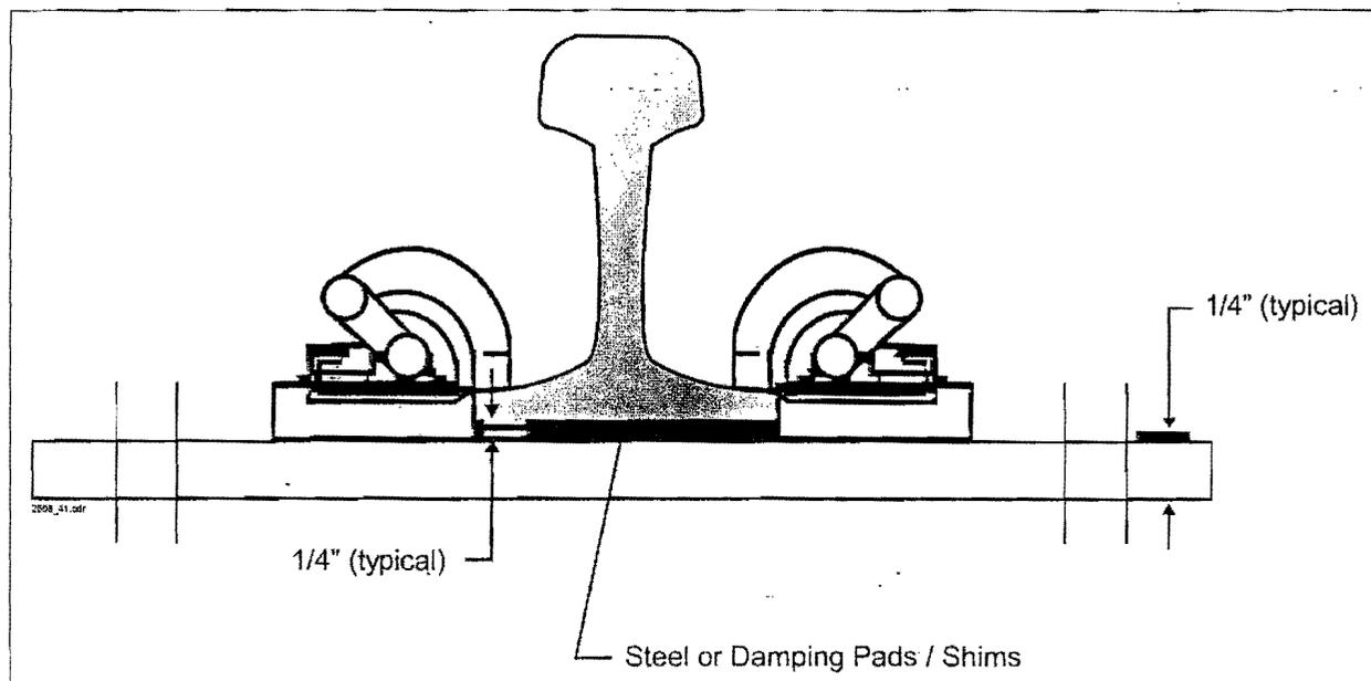
**Figure 41. Cross-Section Sketch of Rail Seat & Pad**
