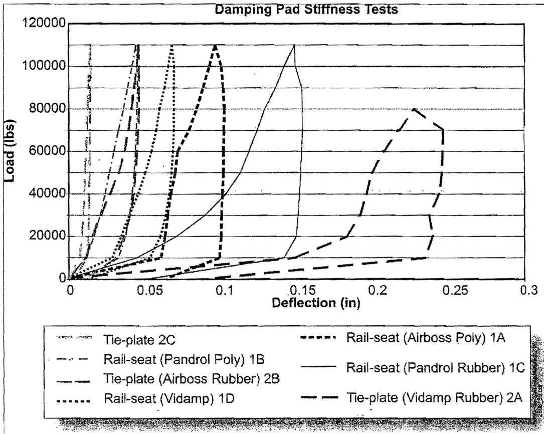
**Figure 39. Typical Load-Deflection-Hysteresis Curve for a Pad**
