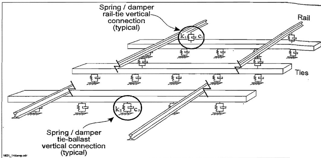
Figure 17. Two-layer NUCARS Track Model for Vertical Vibrations
