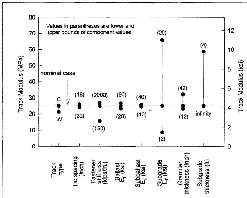
Figure 9. Effects of Track Components on Track Modulus
