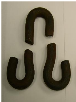
Figure 5. Parts of a NorFast Rail Clip Broke at 70 MGT
