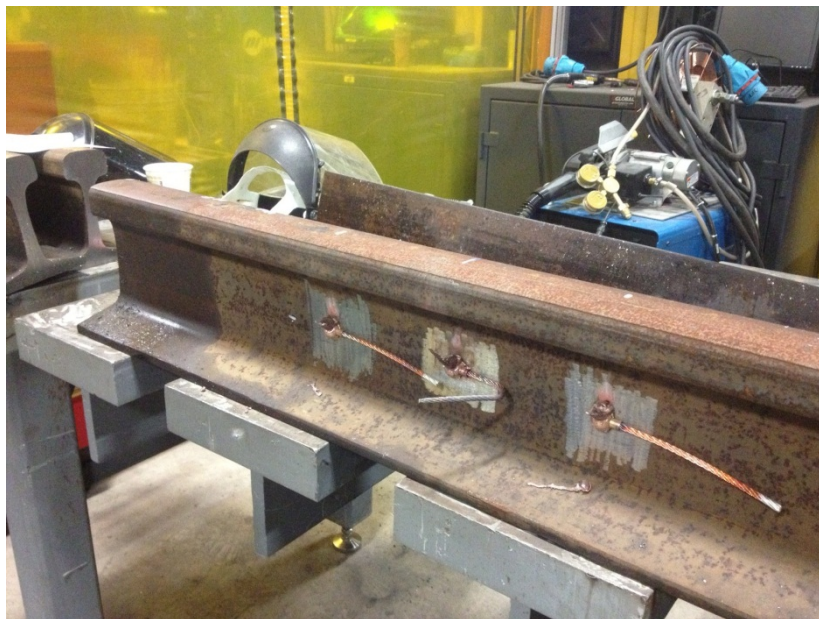
Figure 41. CAD Joint Prior to Corrosion Testing
