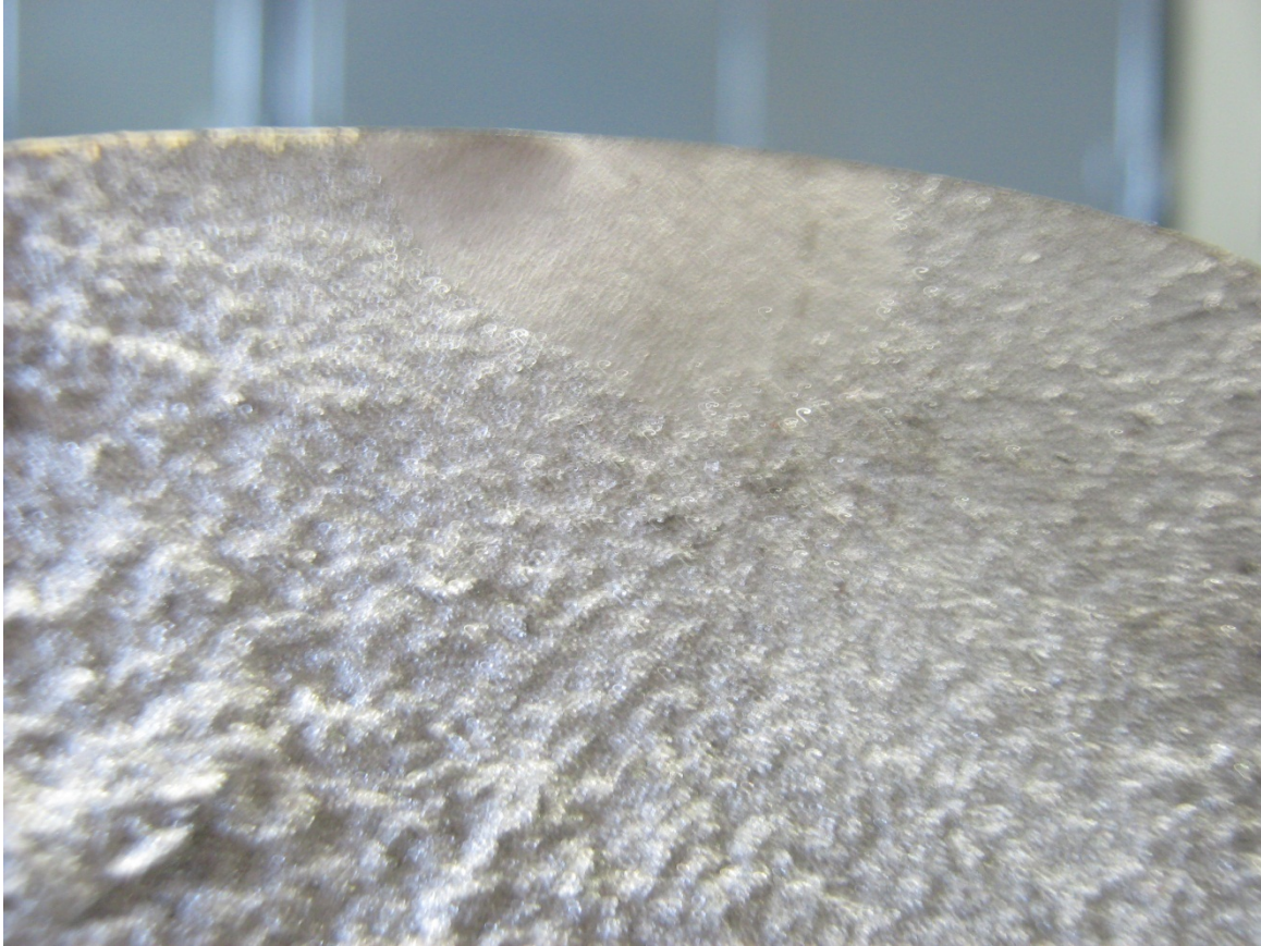
Figure 47. Fatigue Failure Driven by Surface Pitting on Rail Head
