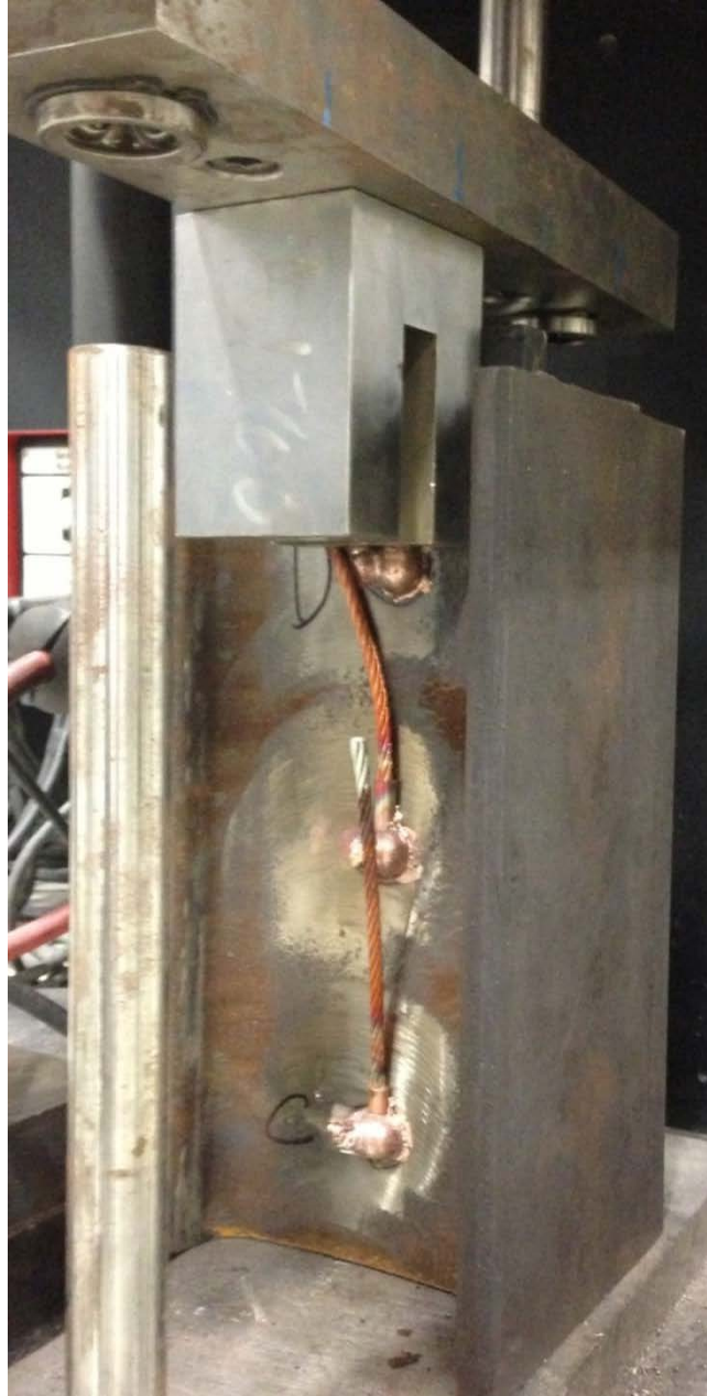
Figure 54. Impact Fixture Applied to CAD Joint
