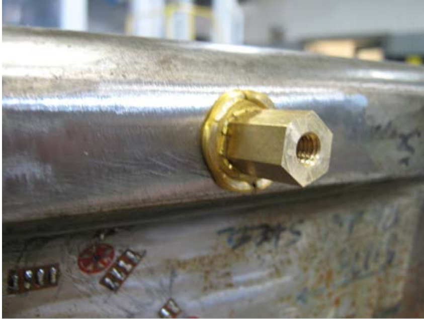
Figure 40. IFW Joint Prior to Corrosion Testing
