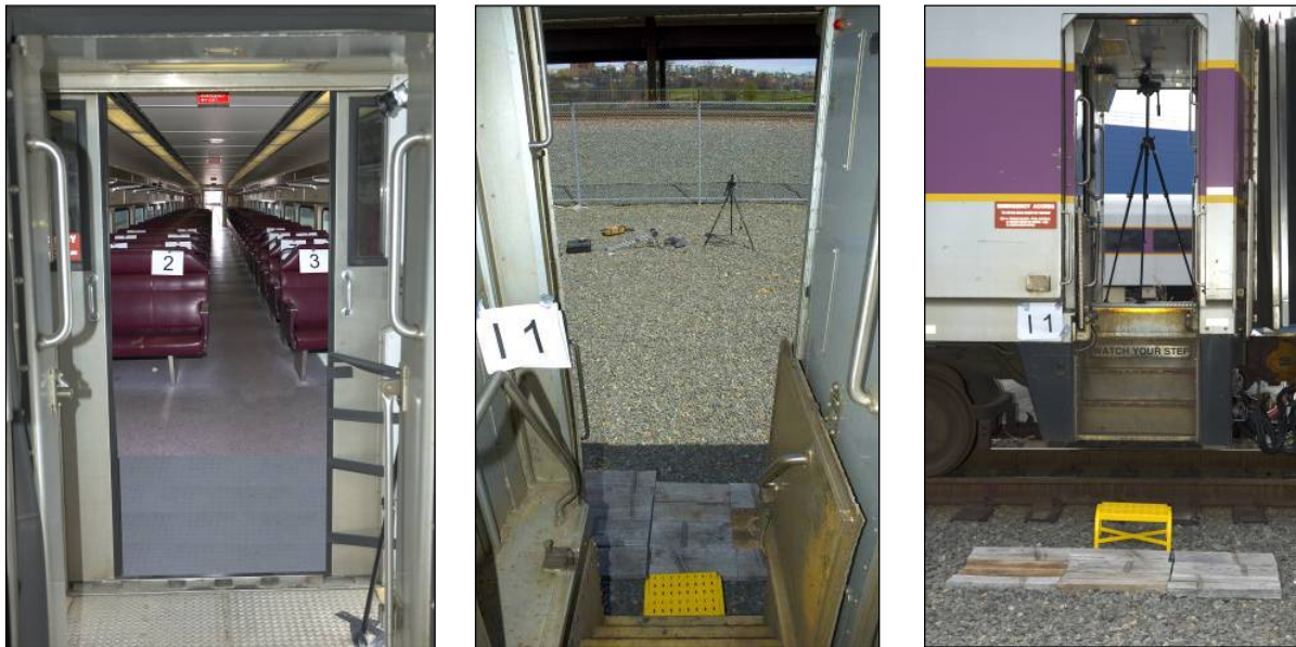
Figure B3. Exit to R-O-W: Passenger Rail Car Interior View and Yellow Step Box / Wooden Pallet and Ballast / Ground Step Area
