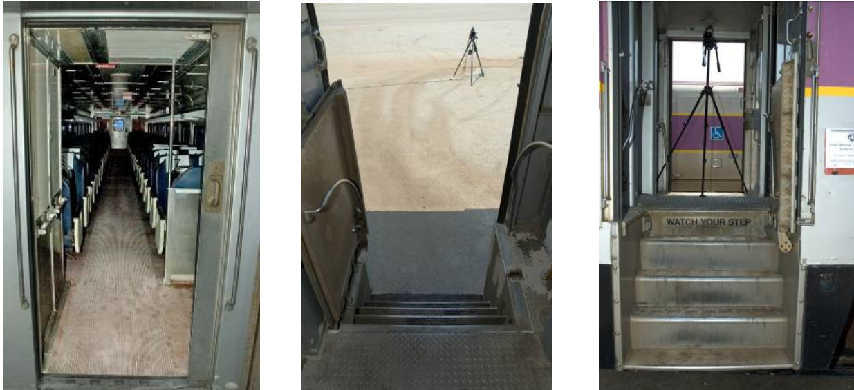
Figure B7. Exit to Low Platform: Passenger Rail Car Interior and Side-Door Exit
