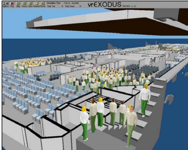
Figure 4. vrEXODUS Output for Large Passenger Ship Generated Using maritimeEXODUS
