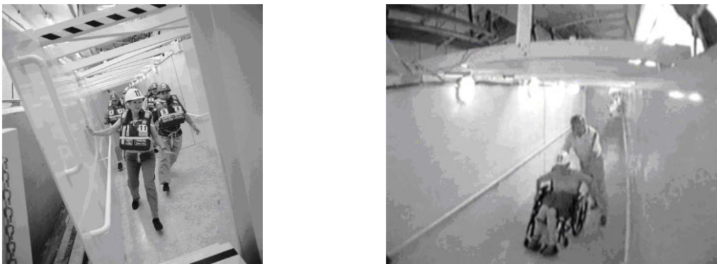
Figure D2. SHEBA Facility Heeled at 20° with Group Evacuation (left) and with Wheelchair Participant Negotiating a 20° Heel
