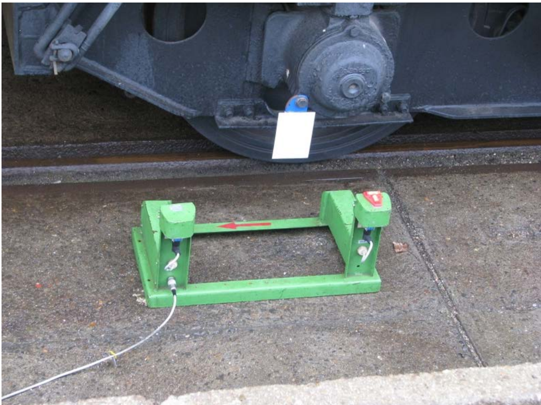
Figure 54. Stroke measurement with photo sensors
