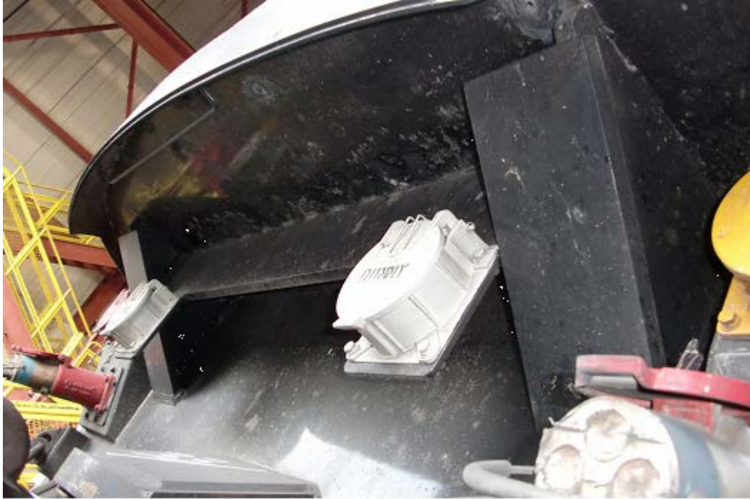
Figure 6. Photograph showing the heavy gusset plates on the forward end of an MP36 locomotive
