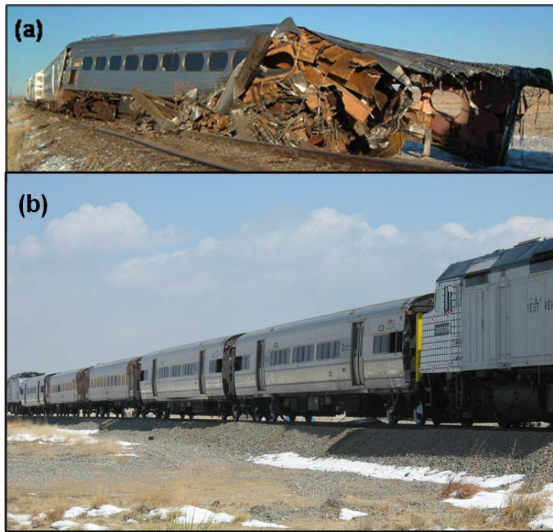
Figure 2. A comparison of the outcomes of full-scale collision tests for: (a) a conventional passenger train and (b) a CEM-based passenger train.
