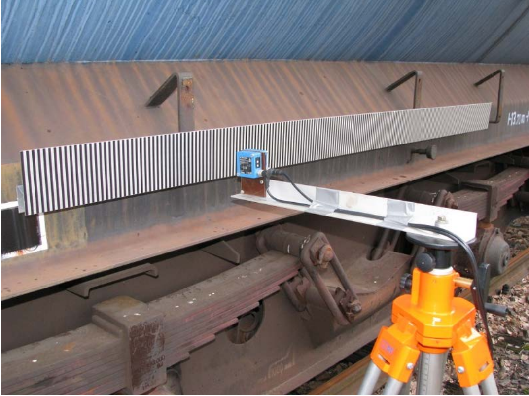
Figure 53. Stroke measurement with laser & ruled strip
