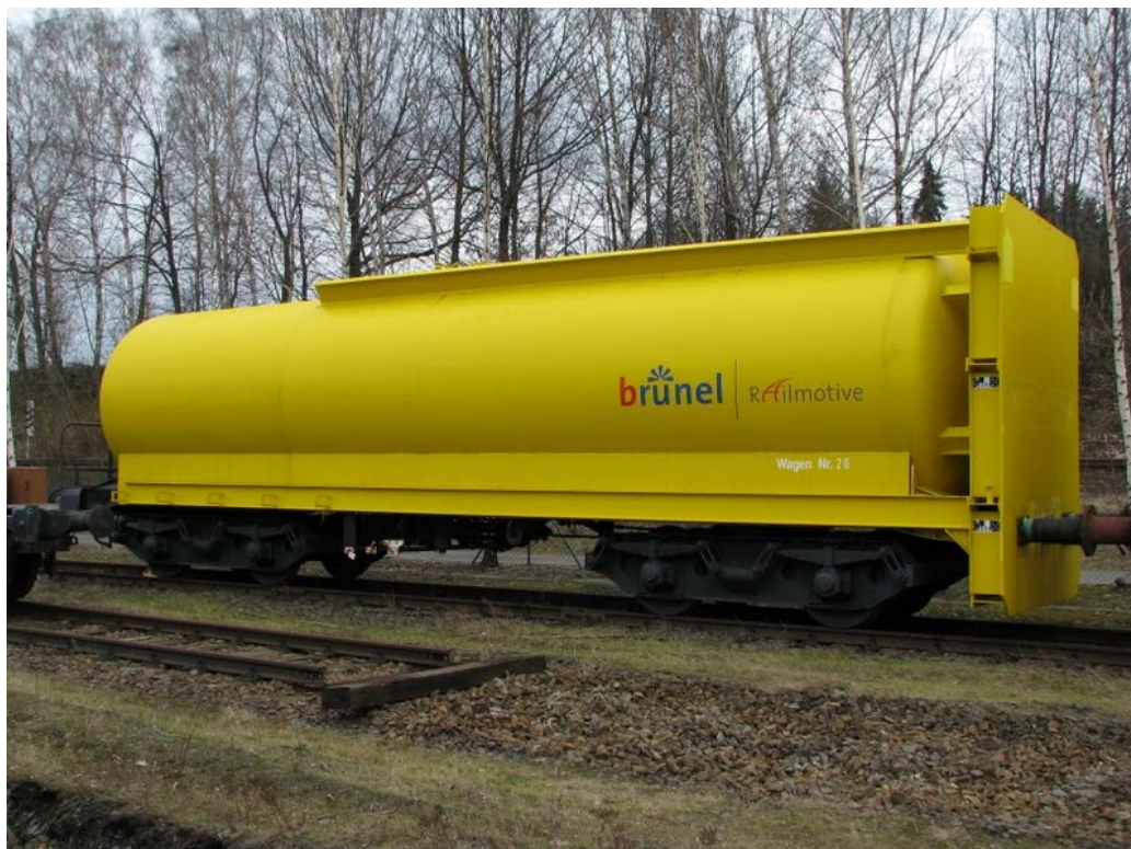
Figure 49. The 78-metric-ton impacting rail car
