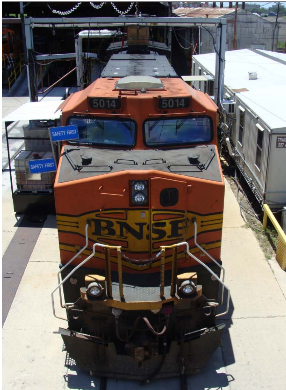
Figure 7. BNSF5014, a Tier 1 Plus GE Dash9-44CW
