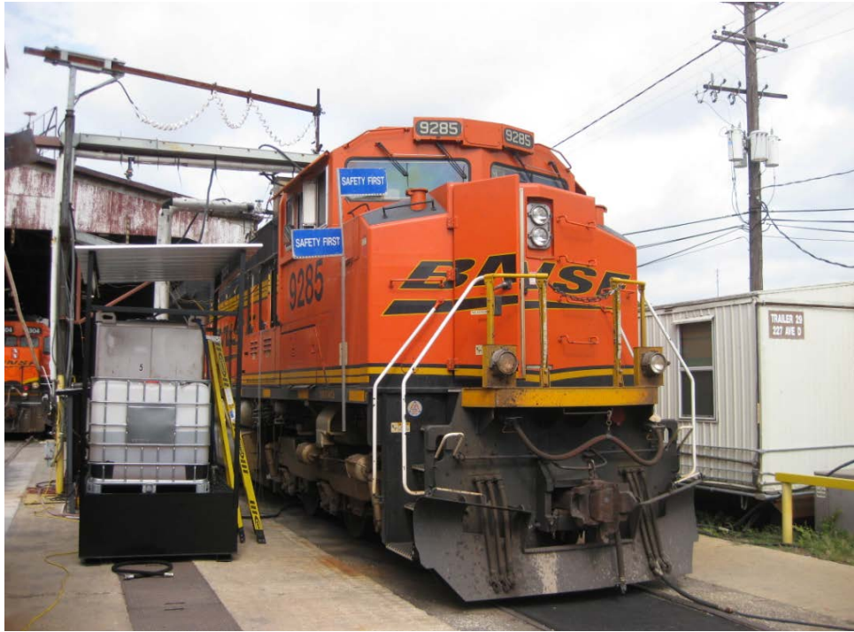
Figure 5. BNSF9285, a Tier 2 EMD SD70ACe
