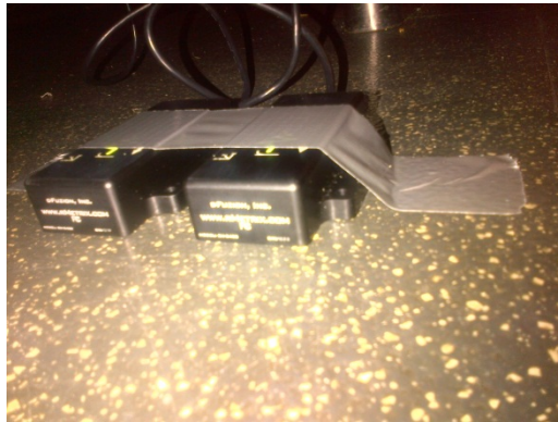
Figure 20. Close-up view of accelerometers
