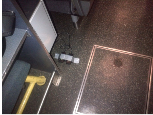
Figure 19. Accelerometers taped down to the floor of Amtrak's geometry car
