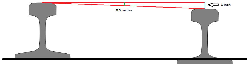
Figure 21. Geometry configuration of data collection with accelerometer
