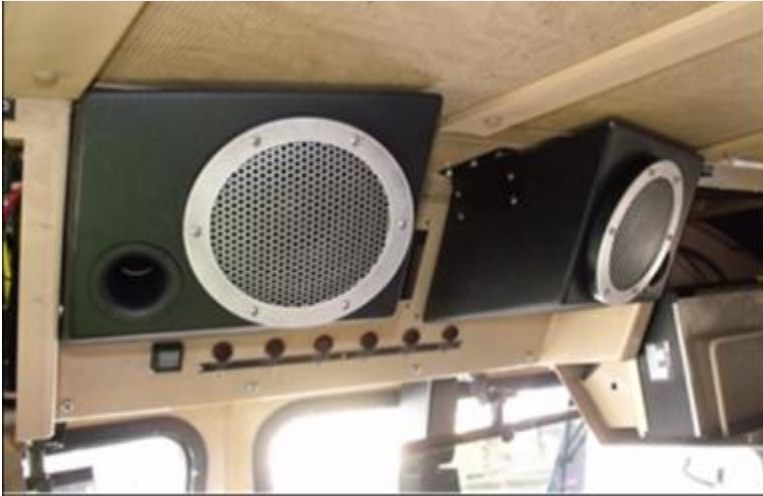
Shown here: Active Noise Cancellation Speakers in Locomotive Cab
