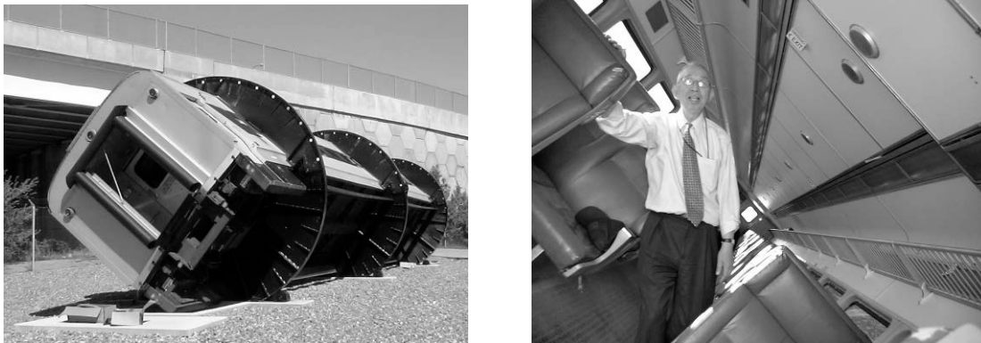
Figure 29. FRA Rollover Rig Exterior and Interior: 45 Degree Angle
