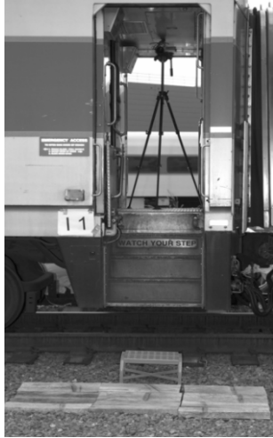
Figure 15. Car #237: Side-Door Stairway – Interior and Exterior Video Cameras
