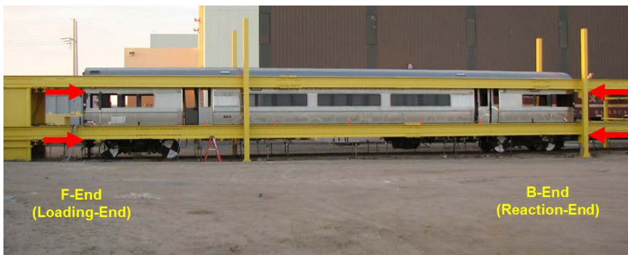
Figure 2. Test car in loading fixture. Arrows indicate approximate location at which loads are applied for crippling load test.
