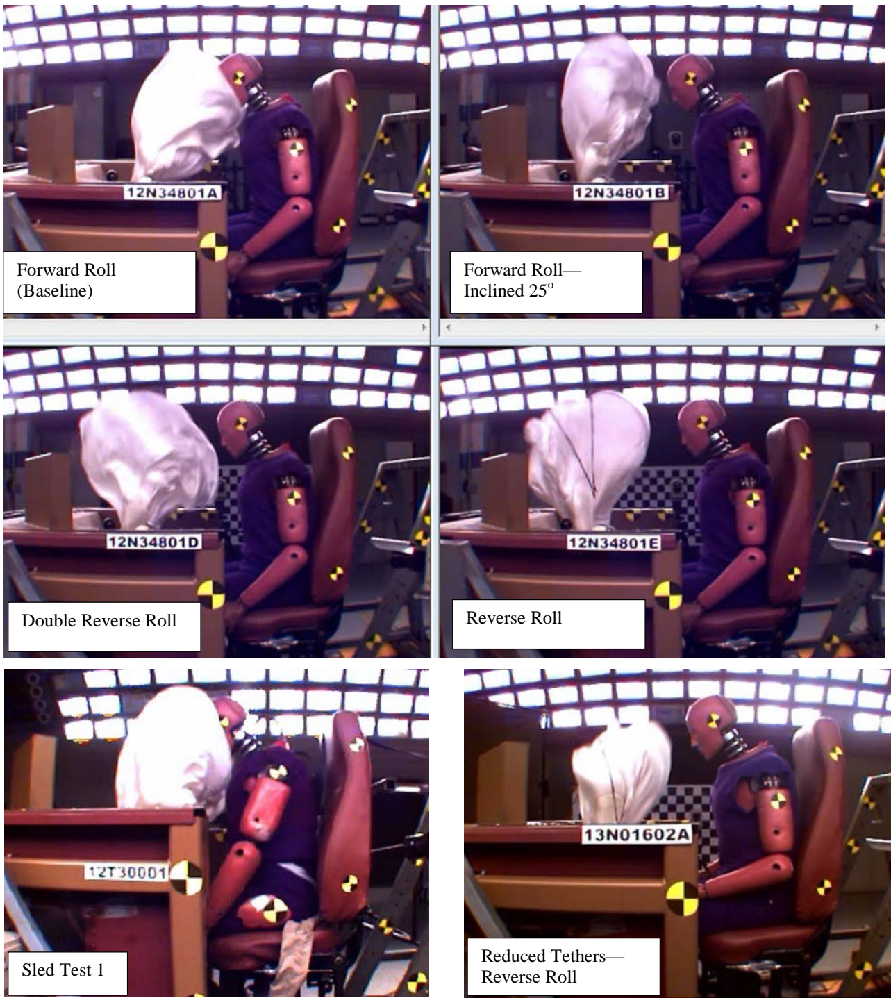
Figure A3. Deployment Sequence—Static Deployment Tests, t = 20 ms
