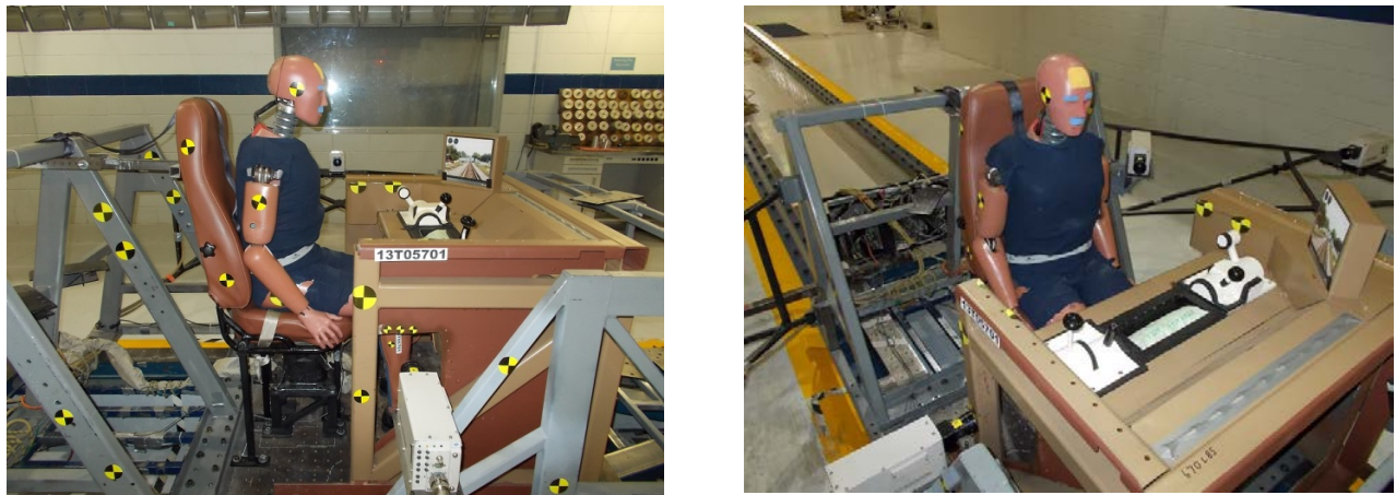
Figure 20. Sled Test Setup—Second Test
