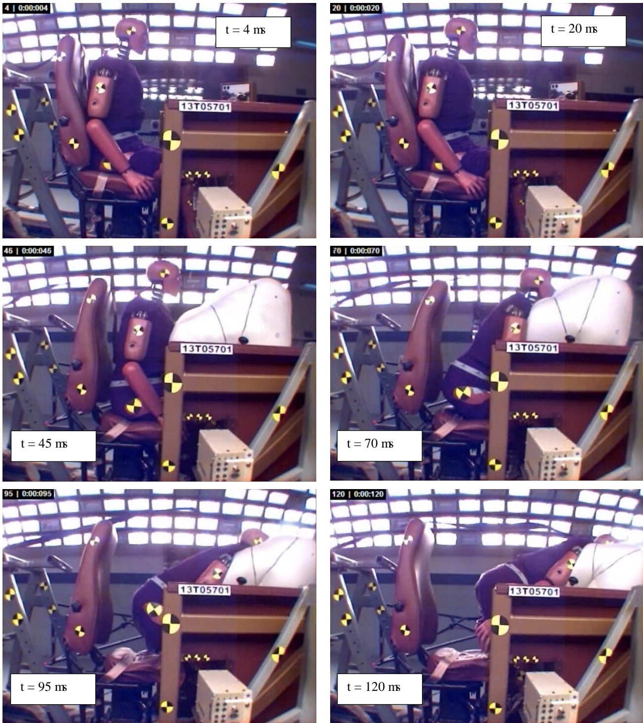
Figure 21. ATD Kinematics from Sled Test—2
