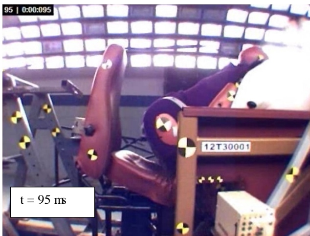
Figure 18. ATD Kinematics from Sled Test - 1
