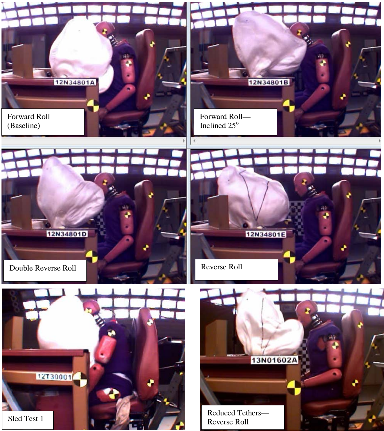
Figure A5. Deployment Sequence—Static Deployment Tests, t = 30 ms
