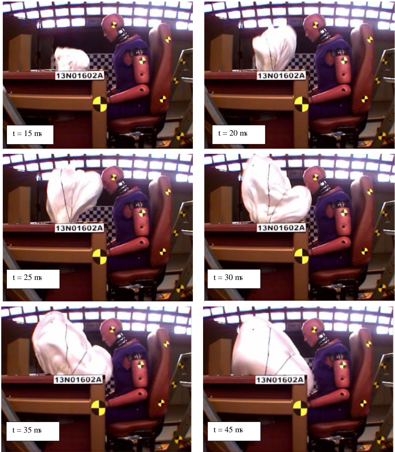
Figure 19. Airbag Deployment Sequence – Reverse Single Roll with Shortened Tethers
