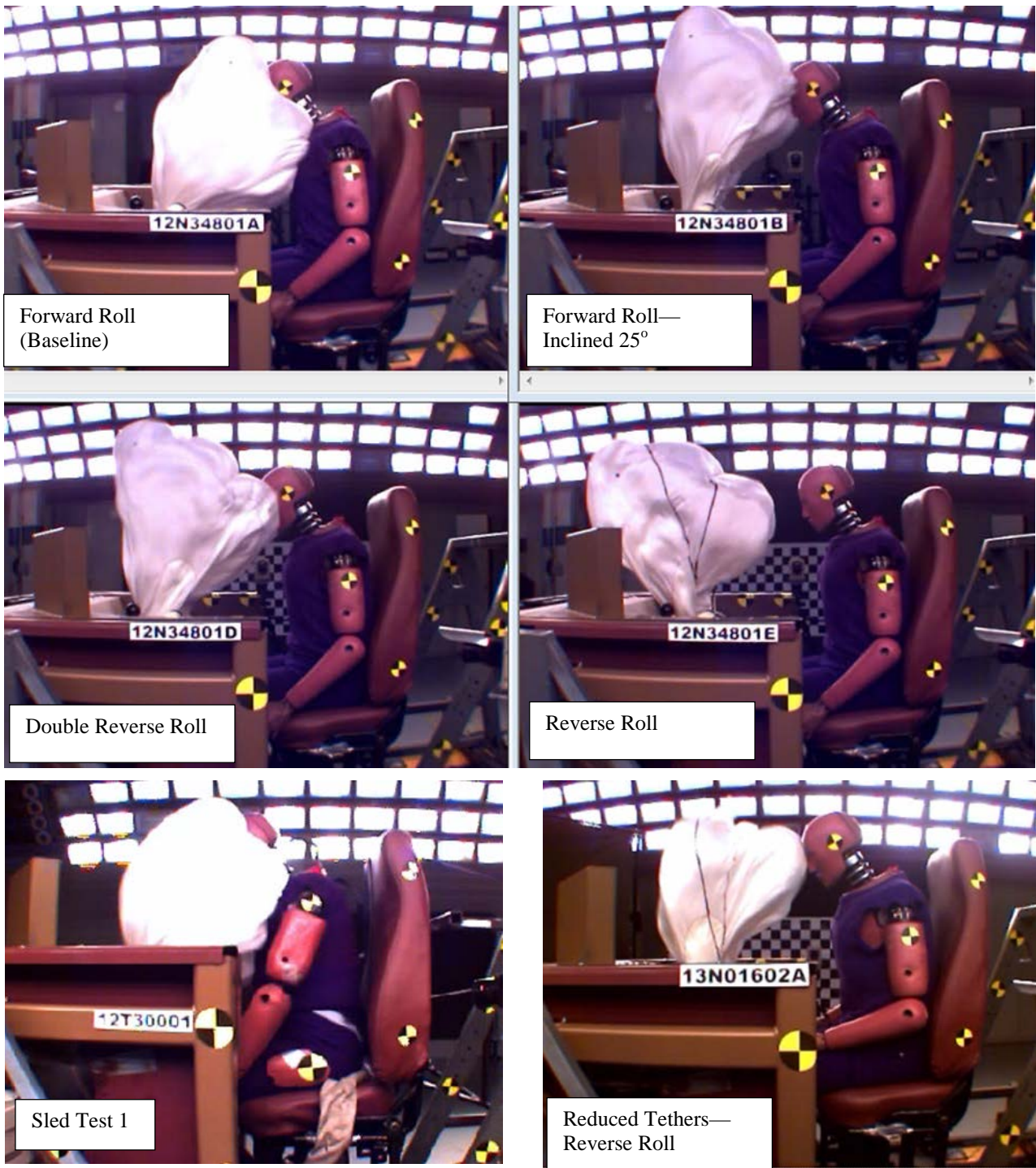
Figure A4. Deployment Sequence—Static Deployment Tests, t = 25 ms
