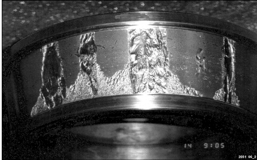
Figure 8. Large Cone Defect in Bearing from Axle 19 of Test Run 24
