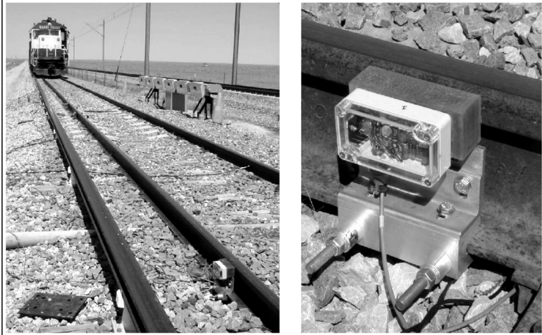
Figure 7. FRA Test Train and Encore Electronics, Inc. Wheel Size Monitor
